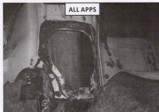
27. Deburr edges and remove loose or excess material from tunnel under where base plate fits.
