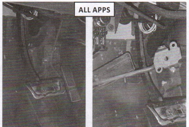
23. If applicable, remove gas pedal. Lift sound deadening from floor to access grommet.
