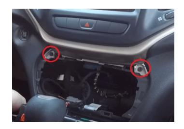
**Step 3:** The radio bezel is now only held in with retainer clips. With a firm pull or using your pry tool, free the radio bezel.
