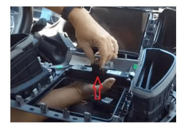
**Step 5:** If you are going from the RA3 to RA4 or from the UAA 5" to the RA3 8.4" or RA4 8.4" the process is the same. Only difference is you may need a GPS and/or XM antenna when going from 5" screen to 8.4" screen upgrade. Remove the four 7mm screws from around the factory radio.
