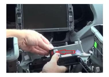
**Step 11:** Push the radio bezel back into place. You'll hear the retainer clips engage to secure the bezel in place.
