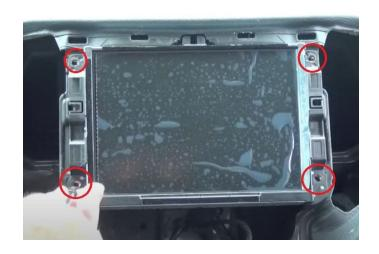
**Step 9:** Next you will need to swap your Hazard button from your 5" bezel over to the new 8.4" bezel. If you already had a RA3 and are upgrading to the RA4 you can skp this step. There are four T15 screw, remove them then move the Hazard button to the 8.4" bezel. Use the same four T15 screws to secure the hazard button in place.
