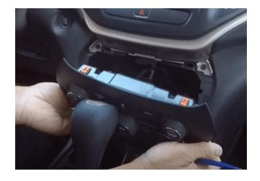
**Step 2:** With the HVAC controls removed, you'll see two 7mm screws to remove from the radio bezel.
