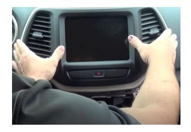
**Step 12:** Reinstall the two 7mm screws to secure radio bezel in place.
