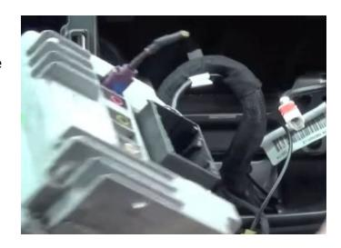
**Step 8:** Place new RA3/RA4 in the dash and secure with the four 7mm screws.
