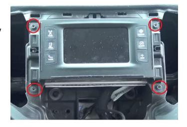
**Step 6:** Lean the radio forward and disconnect the connections on the rear of the radio. Place radio off to the side.
