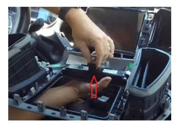
**Step 12:** Remove the four 7mm screws from around the factory radio.
