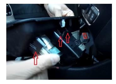
**Step 5:** Slide the new USB hub into place, you'll hear the plastic tabs snap into place.
