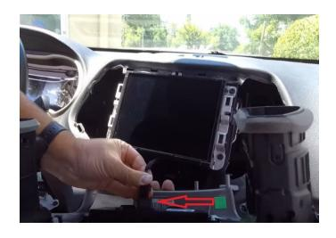
**Step 18:** Push the radio bezel back into place. You'll hear the retainer clips engage to secure the bezel in place.
