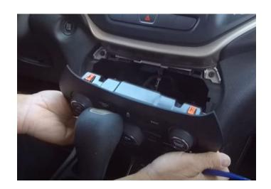
**Step 9:** With the HVAC controls removed, you'll see two 7mm screws to remove from the radio bezel.
