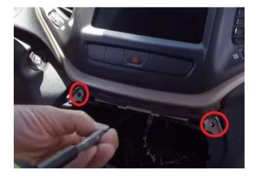
**Step 20:** Reinstall the HVAC controls. They are only held in with retainer clips. Firmly push till you hear the retainer clips engage.
