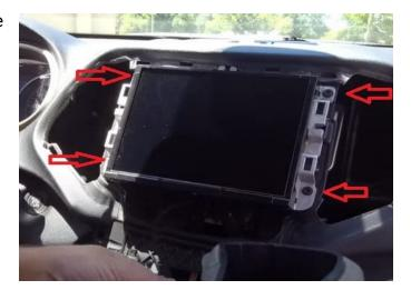
**Step 17:** Next take the radio bezel and plug in the hazard button back in.
