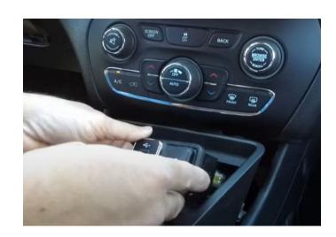
**Step 6:** Plug in the USB hub and the 12 volt outlet. Black USB connector goes on top as the gray USB connector goes on the bottom.
