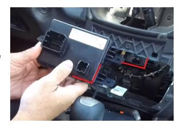
**Step 15:** Take the new UAQ and plug in all the connections that were originally plugged into your factory radio.
