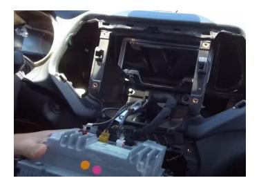
**Step 14:** With the radio removed, you will have access to the factory HVAC module. There are three 5.5mm screws holding the factory HVAC module in place. Remove all three, swap to the new HVAC module then resecure with the same three 5.5mm screws.
