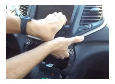
**Step 11:** Lean the radio bezel toward yourself to gain access to the Hazard button connector. Disconnect the hazard button and place bezel off to the side. Be careful to NOT scratch your bezel by placing it face done.
