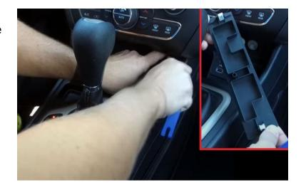
**Step 2:** Next remove the trim panel from around the gear shifter. You don't need to fully remove the panel. Put the emergency brake on then put the vehicle into drive so you have enough room to get to the rear of the factory USB hub.
