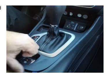
**Step 3:** Disconnect the factory USB hub connections.
