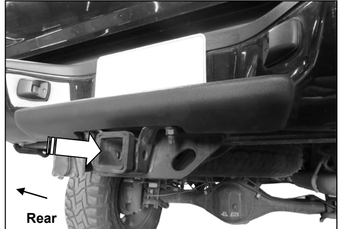
(Fig 2) Insert the tube end on the Hitch Step through hitch opening
