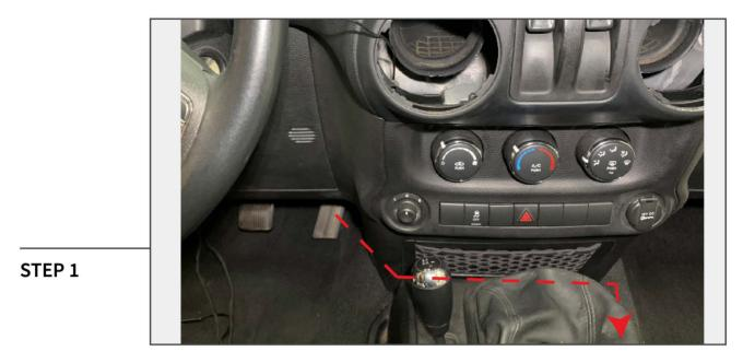
Lay (2) LED Strips in front of each front seat and along the rear seat area. Route the wiring for the rear seat in between the passenger seat and the center console.
