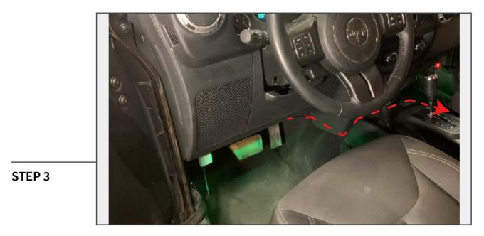
Route the remaining LED Strips towards the rear of the vehicle. Tuck the wiring neatly along the interior trim panels.
