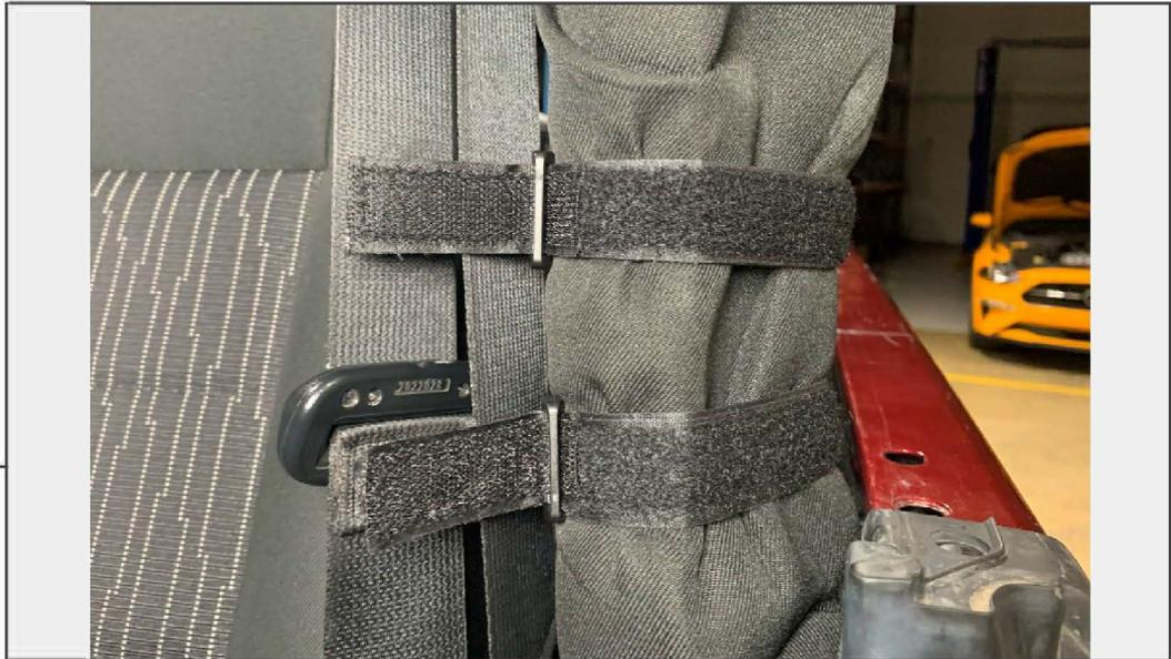
Locate a suitable mounting location along the roll bar. Avoiding any moving components, wrap the straps around the roll bar. Run the straps through the attached clips.
