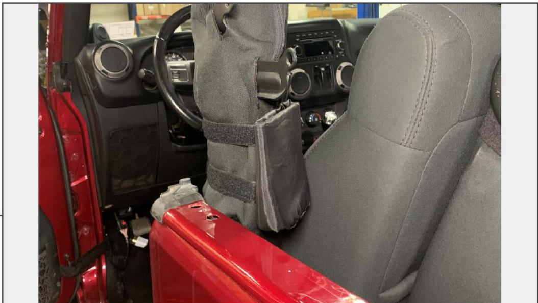
Tighten the straps to secure the drink holder in place.
