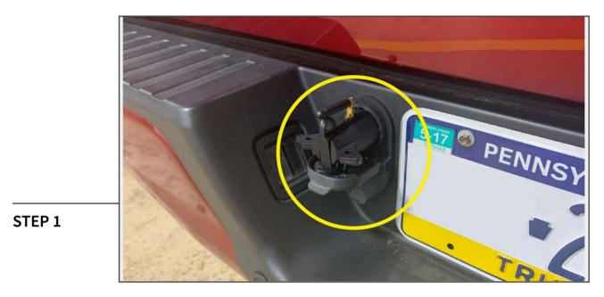
Plug in the vehicle connector into the vehicle's trailer light connector.
