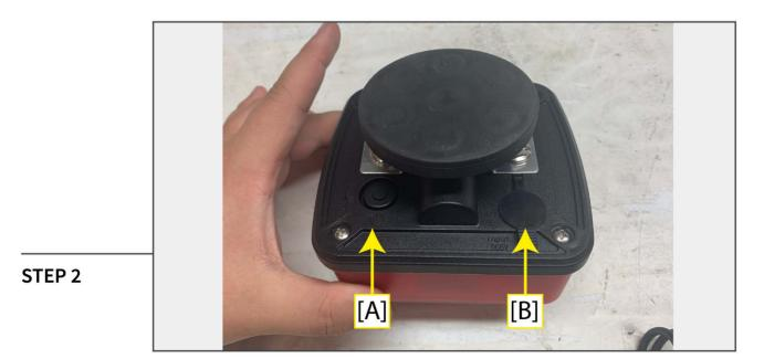
Press the "Power" button on each light [A], then place them at the desired location on the trailer. Test the lights using the turn signals to ensure they are placed on the correct side of the vehicle. \*\*Always test the lights before driving. Charge as needed.
