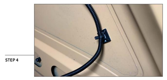
Neatly route the wiring towards the vehicle battery. Using the provided cable tie adhesive mounts and cable ties, secure the wiring harness to the underside of the hood.
