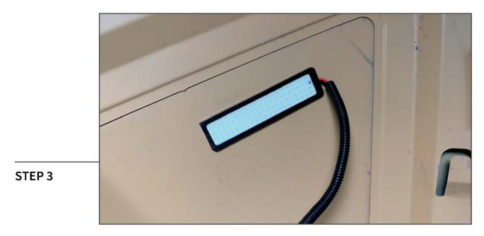
Adhere the LED underhood lights to the desired location by peeling back the double sided tape backing, and pressing the lights firmly into place.
