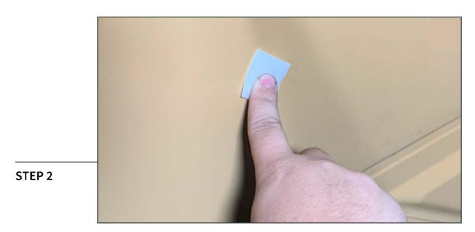
Identify the desired location for the LED underhood lights to be adhered to the vehicle. Clean the desired areas using the provided alcohol wipes.
