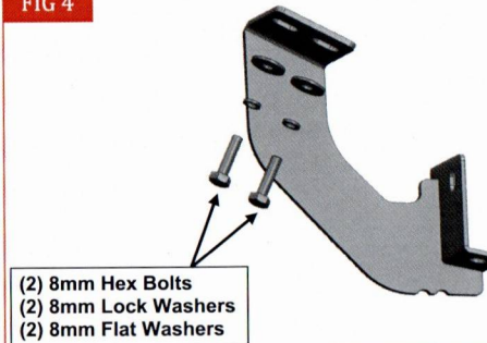
(Fig 4) Attach Driver/Left Center & Rear Mounting Bracket to the floor panel
