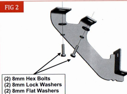
(Fig 2) Attach Driver/Left Front Mounting Bracket to the floor panel
