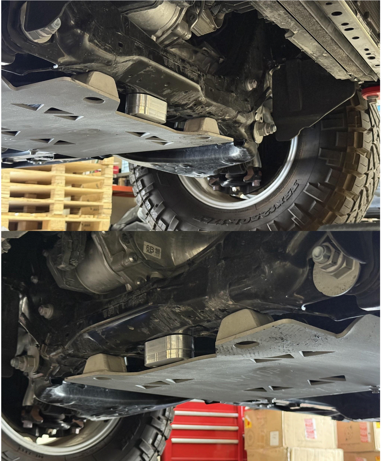
Images showing where the jacking block sits in relation to the middle skid plate.
