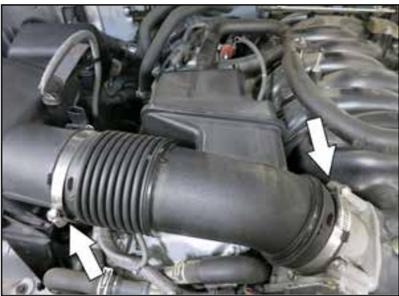
5. Loosen the hose clamps that secure the factory intake tube to the throttle body and air filter housing and remove intake tube.
