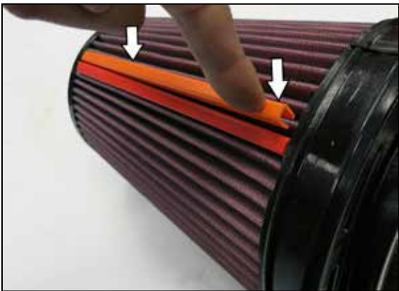
11. Attach the filter clips to the pleats on the air filter align and push down. Passenger side filters, place orange clip on top and red on bottom.
