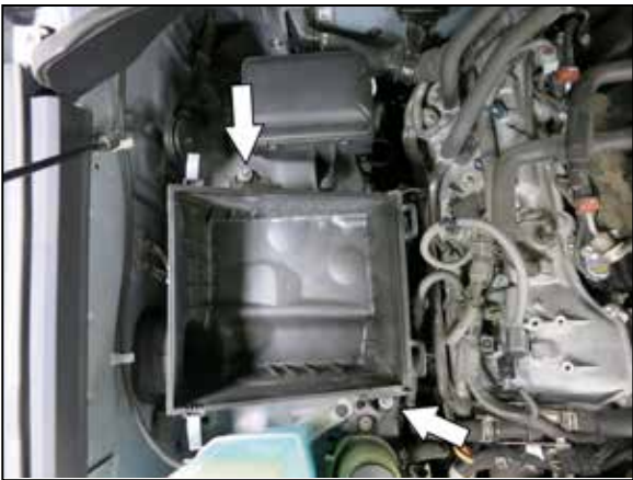
6. Release the latches that secure the upper air filter housing and remove the housing and factory air filter. Loosen the bolts that secure the lower housing to the inner fender and then remove the lower housing from the vehicle.
