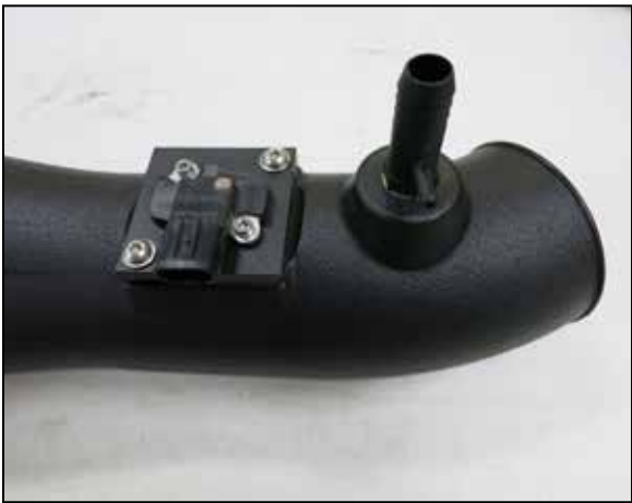
8. Remove the mass air sensor from the factory housing and install it into the K&N adapter using the provided hardware. Install the provided 1/4npt vent fitting into the K&N intake tube as shown. Note: With K&N adaptor on the leftside, make sure the smaller port is facing towards you, as in the photo. Do not over tighten the npt fitting.
