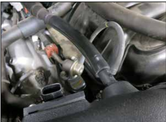
15. Attach the CCV hose assembly to the factory CCV hose and secure the factory spring clamp, then connect the CCV assembly to the fitting in the K&N intake tube. Connect the fuel pressure vent line to the fitting as shown.
