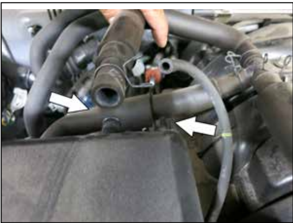
4. Disconnect the CCV hose and fuel pressure vent hose from the factory intake tube.
