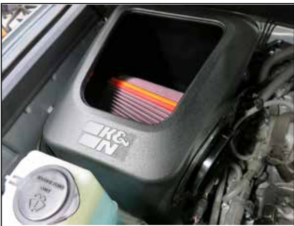
11. Install the K&N air filter into the air filter housing.
