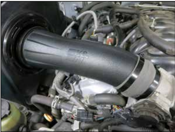
14. Install the K&N intake tube into the filter and attach to the throttle body using the provided coupler and clamps. Adjust the tube for best fit and secure the clamps. Tighten clamps using 5/16" socket or nut driver. Note: Do not over tighten clamps.
