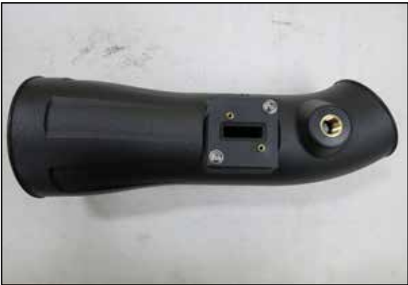
7. Install the mass air sensor adapter onto the K&N intake tube as shown using the provided hardware. Be sure to install the adapter in the correct direction as shown in the photo so the sensor is installed in the correct direction.
