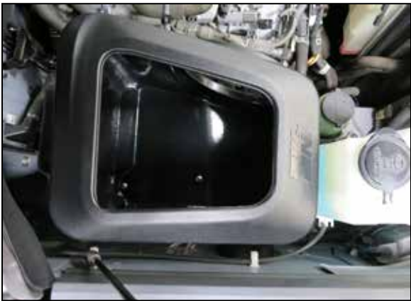
10. Install the K&N air filter housing onto the studs and secure with the provided hardware.
