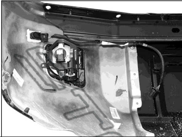
(Fig 16) Remove sensor, fog light and harness
