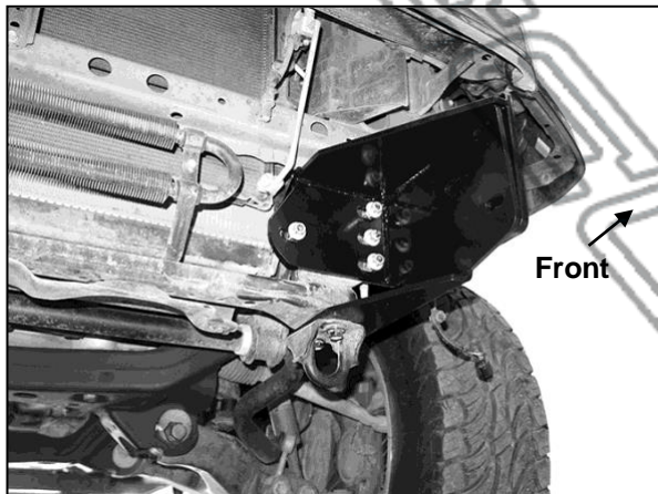
(Fig 13) Support Bracket and Frame Bracket installed
