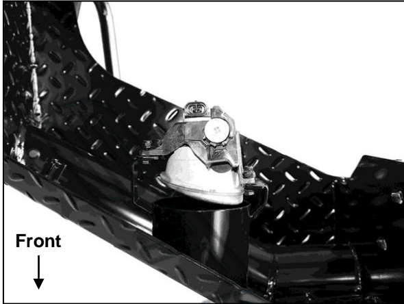
(Fig 21) Driver/left fog light assembly installed
