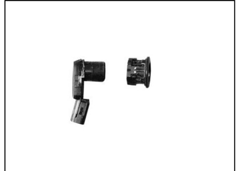
(Fig 17) Sensor and sleeve from bumper
