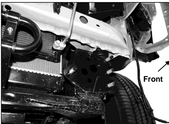
(Fig 10) Bumper removed, driver/left side pictured
