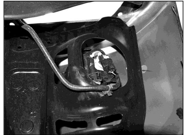
(Fig 7) Unplug wiring harness leading to bumper (passenger/right side pictured)
