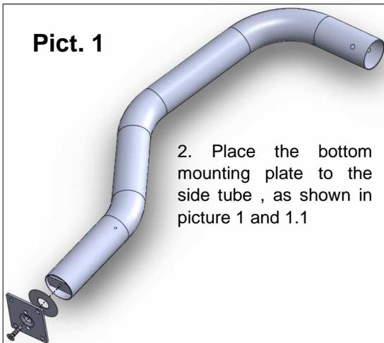
2. Place the bottom mounting plate to the side tube, as shown in picture 1 and 1.1
