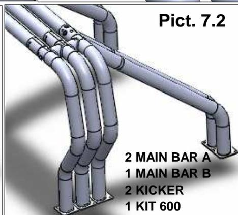
8. Align Bed Bar, and then tighten all bolts, from bottom to up.
