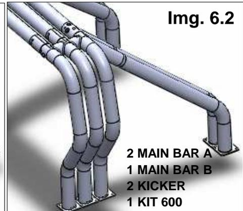
8. Align Bed Bar, and then tighten all bolts, from bottom to top.
