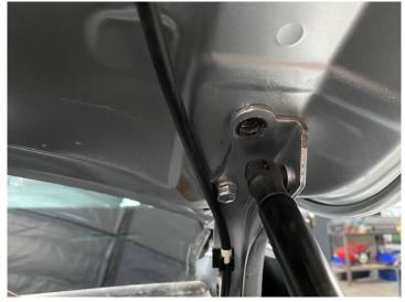
5. Install the ditch light bracket onto the hood hinge bolt, making sure not to pinch the wire on the driver's side. Tighten the bolt up so it is snug but allows the ditch light mount to swing over to complete the installation.
