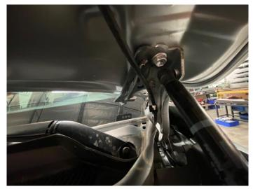
6. Use a socket with a short extension on a ratchet to prevent scratching the paint in the area to remove the lower bolt. For 5" and lights to reduce vibration, rubber trim is provided to put in between the ditch light mount and the edge of the hood. For applications requiring the trim, slide the trim onto the mount and then the bottom hood mount bolt. Remove the lower bolt for the hood mount on the hinge and swing the ditch light mount to align the holes and re-install the bolt.
