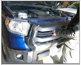
Step 3 Firmly grab and pull factory grille off vehicle. Discard factory grille.
