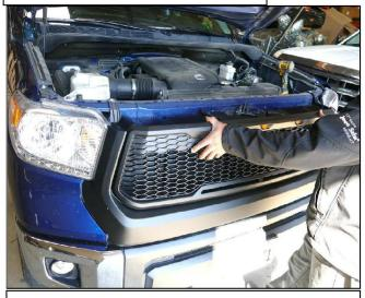
Step 1 Install grille onto vehicle by reversing steps 1-2 in the removal process.
