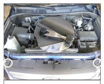
Step 2 Using a plastic clip removal tool or similar tool remove 2 factory clips circled above.
