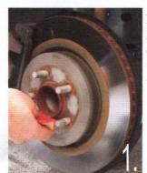
After removal of tires and inspection of rotors, remove any visible rust from the mating flange on the vehicle's rotor. Inspect both the rotor and wheel mounting flanges for burrs, rivet heads, push nut or other obstruction that would prevent a flush seating of the vehicle rotor's mounting flange to both the inner and outer side of the spacer. Improperly seated spacers are hazardous and may cause spacer failure, resulting in the loss of a wheel while driving the vehicle.
