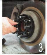
First tighten all lugs to 30 Ft. Lbs. of torque using a star pattern tightening sequence. (see chart below) Once all lugs have been tightened to 30 Ft. Lbs. of torque, continue tightening lugs to the manufacturers torque setting as defined in your owners manual. The table below is for reference only Do not use an impact wrench!
