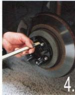
Check for proper tire clearance in the wheel well, making certain there is sufficient wheel and tire clearance for full steering (lock-to-lock). See stud clearance graphic to the right
