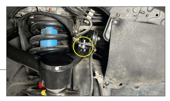
With the vehicle suspension loaded, torque the upper control arm 22mm bolt to 81 ft. lbs.
