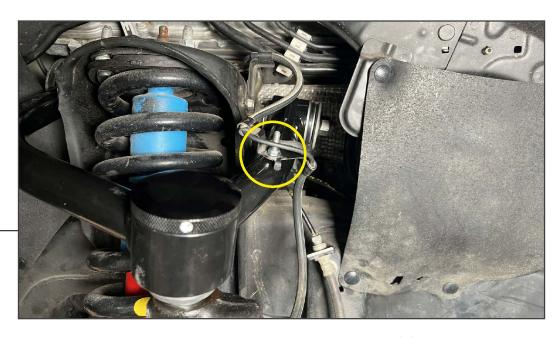
Secure the ABS line bracket to the new control arm stud using the included (1) 10mm lock nut.
