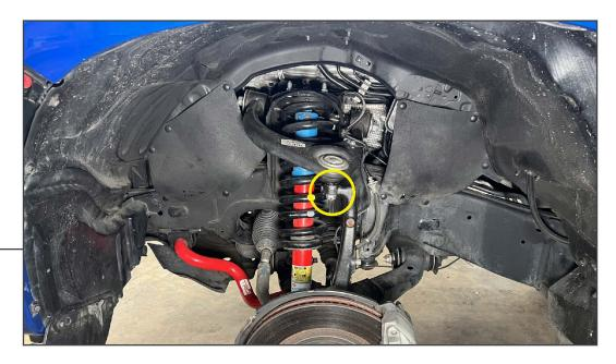
Remove the upper ball joint cotter pin. Then loosen, but do not remove, the (1) 19mm ball joint nut.
