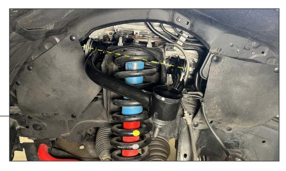
Install the new control arm to the vehicle reusing the original 22mm bolt. Do not fully tighten the bolt at this time. The control arm mounting bolt will be tightened with the vehicle on the ground with the suspension loaded.
