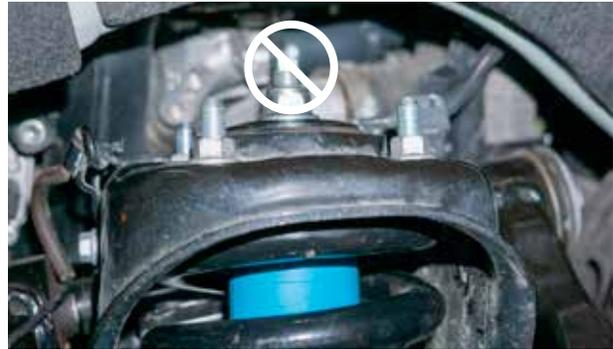
Fig. 4: Remove the four top hat nuts.
