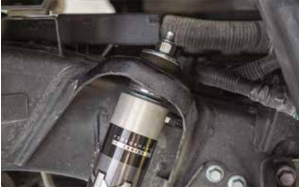
Fig. 12: Install the stem top nut (passenger side shown).
