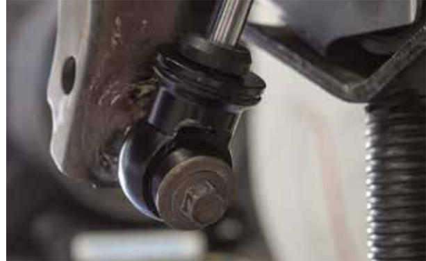
Fig. 13: Install the lower shock bolt (passenger side shown).
