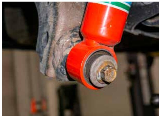
Fig. 11: Remove lower shock mount bolt.
