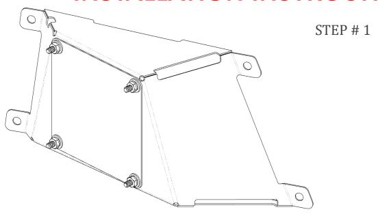
Remove blank plate with 5/32" hex driver and 7/16" drive socket.
