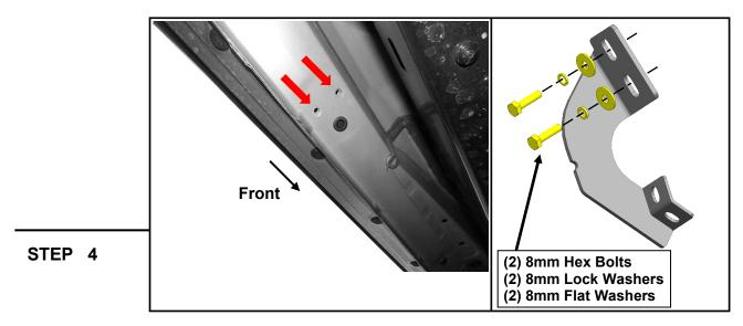
Loosely fit the (1) Driver Center bracket to the vehicle threaded body hole using (2) M8 x 30mm bolts, (2) M8 lock washers, and (2) M8 flat washers. Do not fully tighten to allow for later adjustments. Repeat this step for all Driver Rear brackets.
