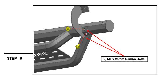
With all brackets loosely mounted to the vehicle, fit the Drop Step onto the brackets, and loosely secure into place using (8) M8 x 25mm combo bolts.
