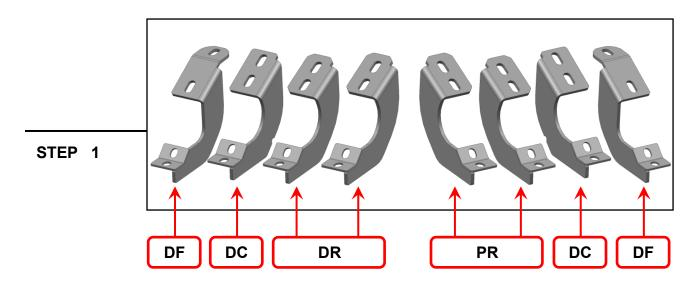
Please identify each mounting bracket using the engraved location identifier. Notice: The center bracket have a notch on the back .The rear bracket per side are interchangeable.
