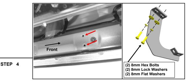
Loosely fit the (1) Driver Center bracket to the vehicle threaded body hole using (2) M8 x 30mm bolt, (2) M8 lock washer, and (2) M8 flat washer. Do not fully tighten to allow for later adjustments. Repeat this step for the remaining Driver Center & Rear brackets.
