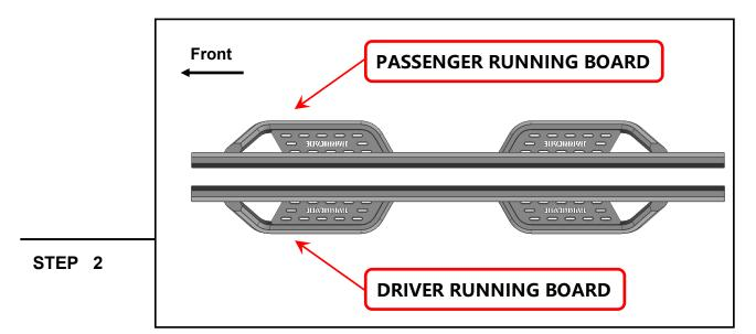
Identify each running board by identifier on the front. Notice: "D" for Driver/Left Side; "P" for Passenger/Right Side.
