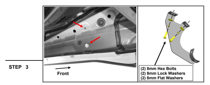
Start installation toward the front of the Driver/Left side of the vehicle.
