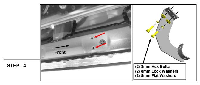
Loosely fit the (1) Driver Center bracket to the vehicle threaded body hole using (2) M8 x 30mm bolt, (2) M8 lock washer, and (2) M8 flat washer. Do not fully tighten to allow for later adjustments. Repeat this step for the remaining Driver Center & Rear brackets.
