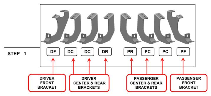
Please identify each mounting bracket using the engraved location identifier. Notice: The center bracket and rear bracket per side are interchangeable.
