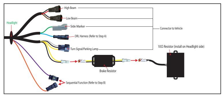
A Connect DRL fuse harness to the lights, and then insert the fuse into the fuse box.
