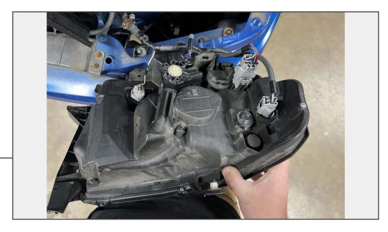
Unplug the electrical connectors from the back of the headlight assembly. Set the headlight assembly aside.
