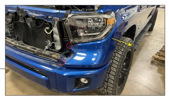
Remove (2) plastic push clips from the painted panel below the headlight assembly. Then, pull the painted trim panel away from the vehicle fender to dislodge the retaining clips. Set the panel aside.
