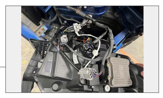
Plug the new headlight into the vehicle wiring harnesses. Plug the DRL harness into the headlight assembly.
