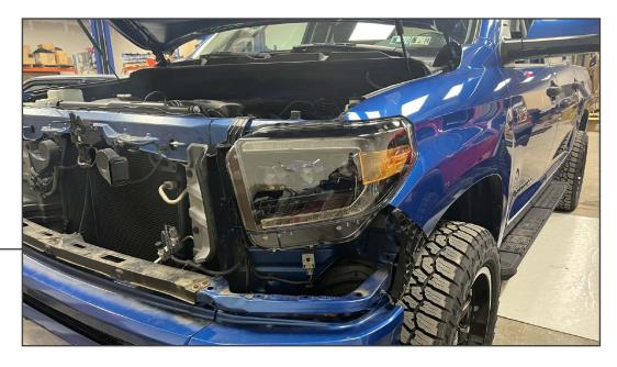
Secure the headlight into the vehicle reusing the original hardware.
