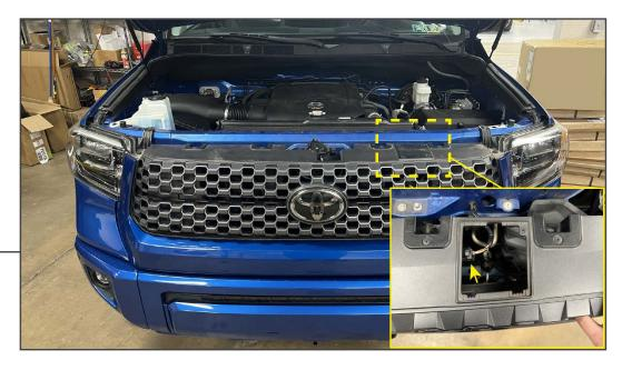
Open the vehicle hood. Remove the small cover on the top of the grille using a pry tool. Unplug the grille electrical connector.
