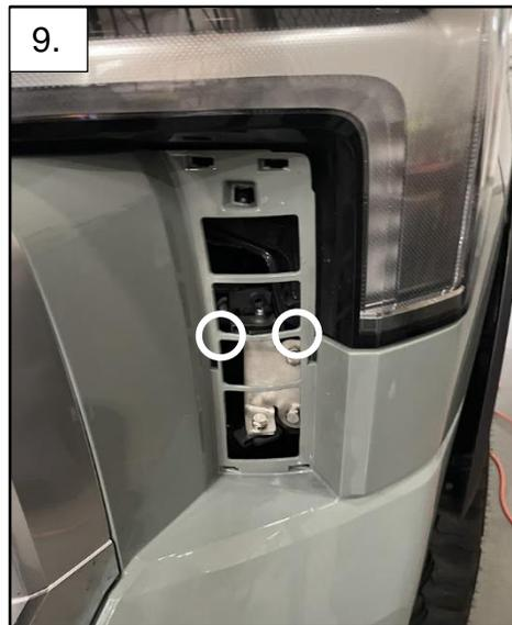
10. Locate the crash attenuator located underneath the driver side headlight. The provided clip-on nuts will be applied into both circled holes.
