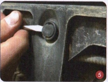
(5) Unclip plastic clips that are holding the plastic step to the top of the bumper.
