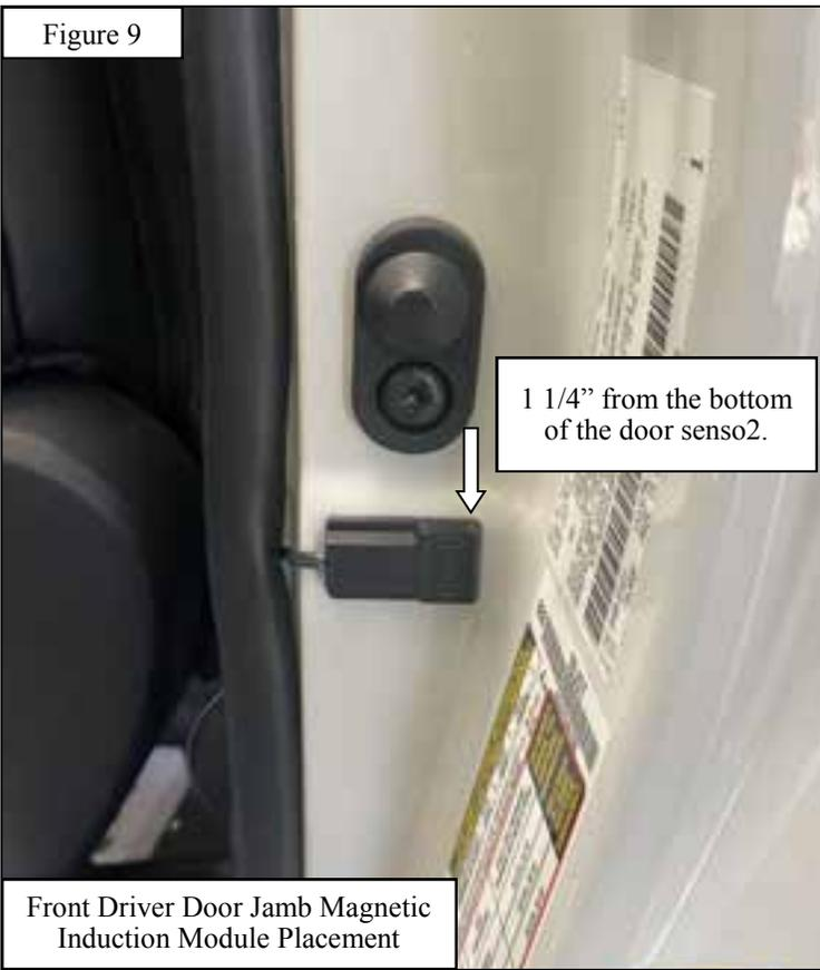
Front Driver Door Jamb Magnetic Induction Module Placement
