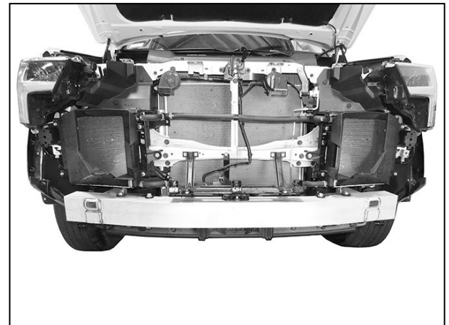
(Fig 8) Grille/bumper cover assembly removed
