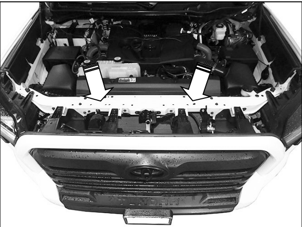
(Fig 7) Remove all hardware attaching top of grille and bumper cover to radiator core support (arrows) and remove grille/bumper cover assembly
