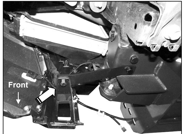
(Fig 44) Attach outer end of Support Bracket to factory bumper (arrow-also see Fig 43). Driver/left side pictured from behind bumper
