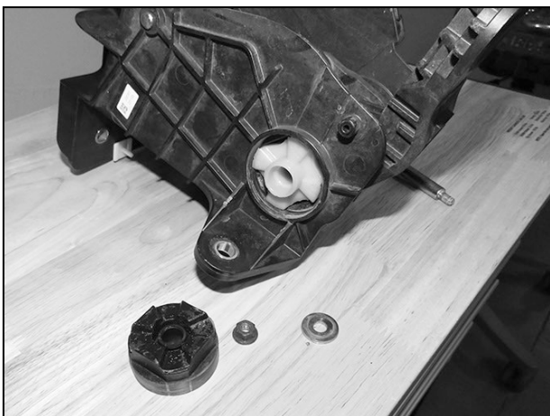
(Fig 14) Remove outer covers and inner drive from both sides
