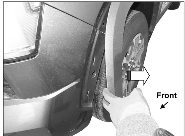
(Fig 2) Models with fender flares, pull end of flare outward to release clips from body
