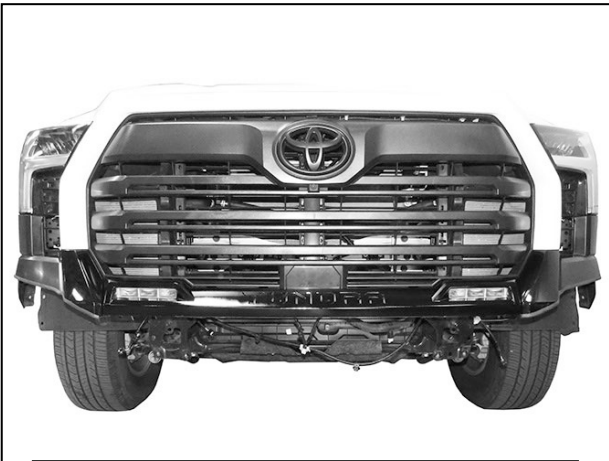
(Fig 44) Reinstall grille/bumper assembly
