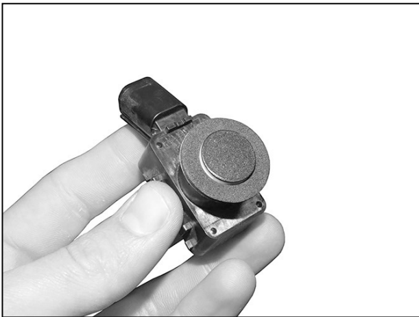
(Fig 49) Apply Foam Seals to end of sensors
