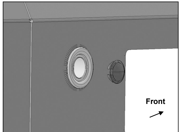
(Fig 45) Models without front sensors, push sensor plugs into mounts
