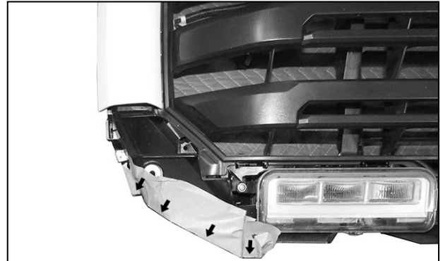
(Fig 42) Inner bumper support cut along tape
