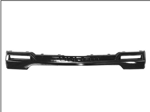
(Fig 32) Center grille body panel (fascia)
