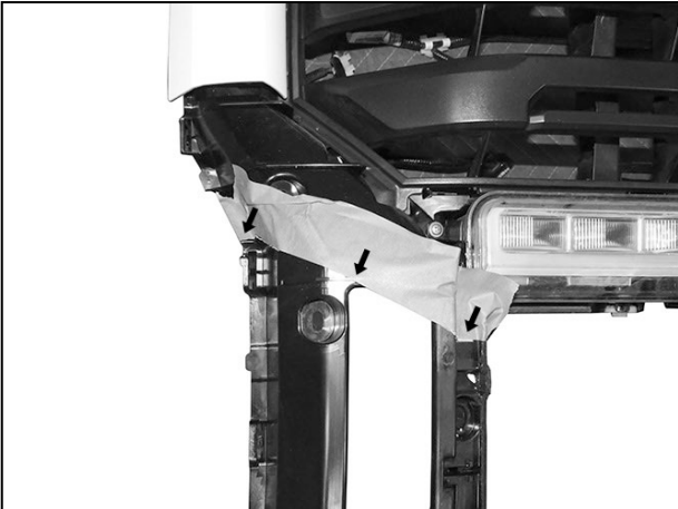
(Fig 41) Use masking tape to make a diagonal guide line along bumper fill panel (see Fig 40) and cut bottom section off of inner bumper support along tape
