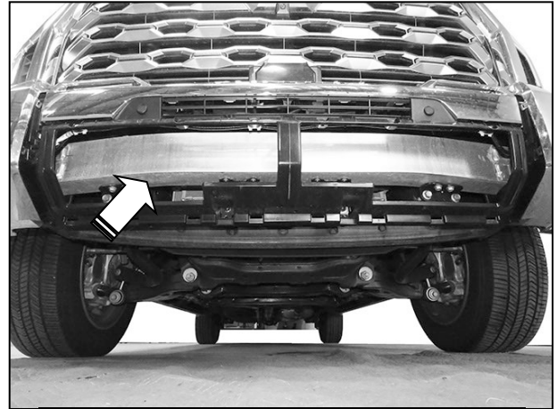
(Fig 4) Remove lower cover from bumper
