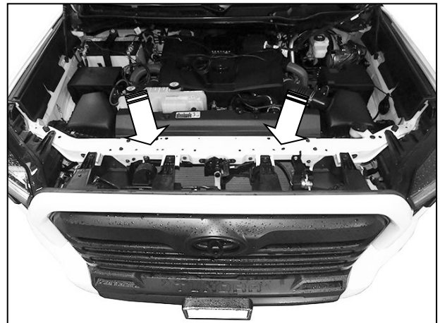
(Fig 6) Remove all hardware attaching top of grille and bumper cover to radiator core support (arrows) and remove grille/bumper cover assembly
