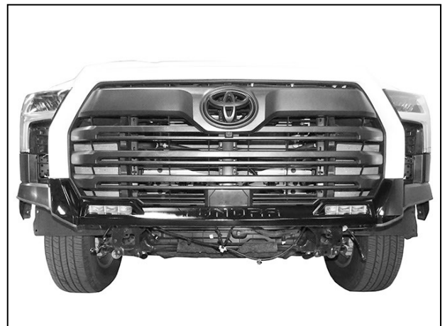
(Fig 44) Reinstall grille/bumper assembly
