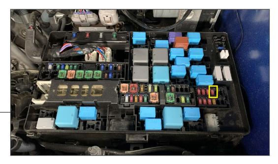
Connect the (1) fuse tap to the Red wire lead. Connect the fuse tap to the vehicle ignition fuse in the fuse box, and route the wiring out of the fuse box. Then, connect the ring terminal to the Black wire lead. Fit the wire lead to the vehicle battery/chassis ground. Route the harness neatly using the included (5) cable ties.
