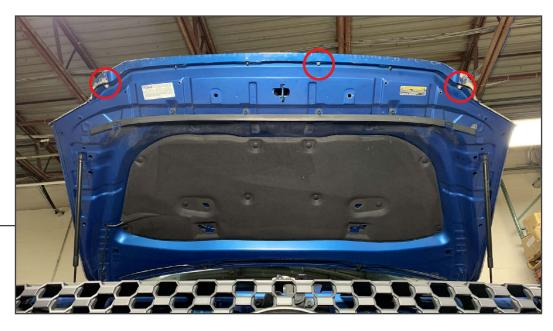
Open the vehicle hood, and locate the hood mounted panel. Remove (3) 10mm bolts from the hood mounted panel.
