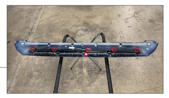
Remove (6) Phillips head screws from the hood mounted panel to remove the panel insert. Remove the panel insert and set aside.
