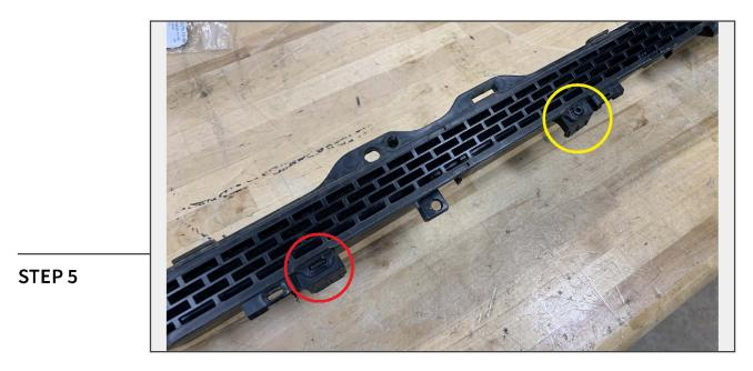
Use a flathead screwdriver and dislodge the mesh from the panel insert perimeter, and use a drill and drill bit to remove the (1) plastic rivet. Remove the mesh insert from the panel.
