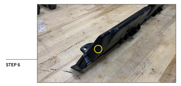
Using a drill and drill bit, drill a hole in the panel insert to route the included wiring harness through from the lights to the inside of the hood.
