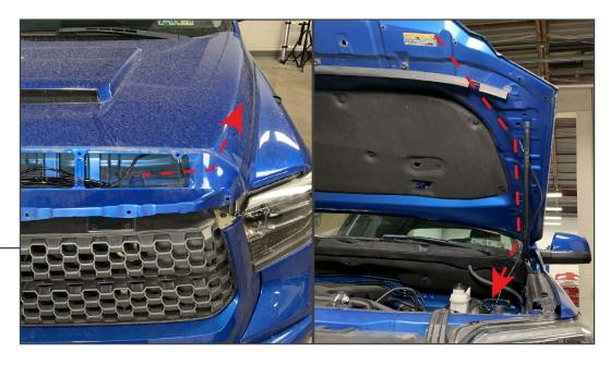
Route the wiring harness through the hood, and have the harness exit through the pre-drilled hole next to the hood strut on the driver's side of the vehicle. Neatly route the harness towards the vehicle fuse box and battery.
