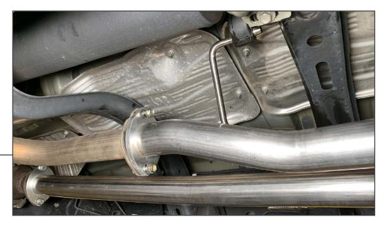
Ensure the original exhaust flange gasket is in place. Install the LH front pipe to the vehicle exhaust using the (2) original 14mm bolts. Insert the welded hanger into the vehicle rubber hanger.
