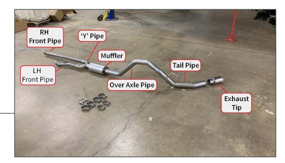
Lay out and identify all exhaust components.
