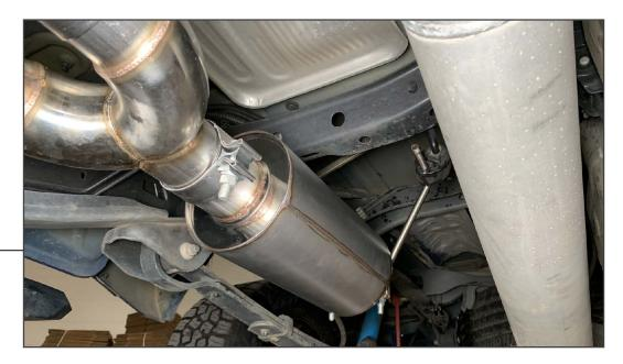
Install the muffler to the 'Y' pipe, and loosely secure using the previously placed 3" exhaust clamp. At the outlet portion of the muffler, place the (1) hanger clamp, and insert the hanger clamp into the vehicle rubber hanger.
