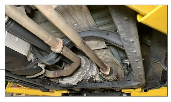
Lift and support the vehicle using a floor jack and jack stands. Locate the LH and RH side exhaust flanges. Remove the (2) 14mm bolts from each exhaust flange. Ensure the gaskets remain on the flange during removal.
