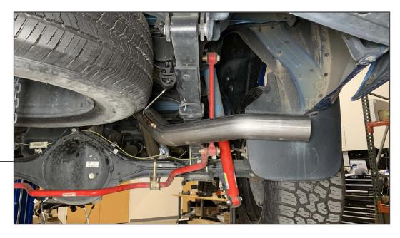
Install the tail pipe to the over axle pipe, and loosely secure using the previously placed 3" exhaust clamp. Insert the welded hanger into the vehicle rubber hanger.
