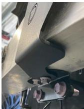
3. Install the base SS5 bracket over the bumper support and secure it using the original bolts removed in the previous step. Ensure the DD logo is in the correct orientation. Do not overtighten the bolts. Repeat this step on the other side of the vehicle.
