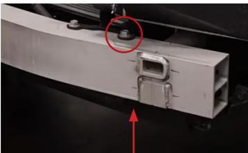
2. Using a 14mm socket, remove the bolt on the bottom side of the bumper support. Then, using a 17mm socket, remove the bolt on the top side of the bumper support. Repeat this step on the other side of the vehicle.
