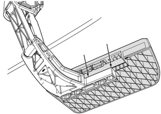
Insert PT Screws (6) into corresponding holes
