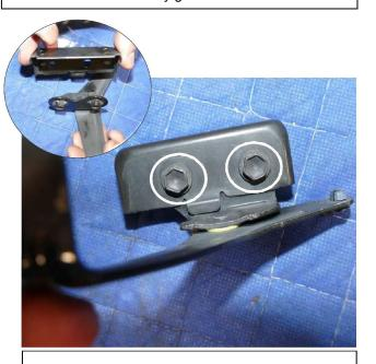
Step 6 Remove factory hood latch from factory bracket by removing 2 factory bolts shown above using a 10mm socket.
