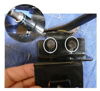
Step 2 Install factory bolts through the mounting bracket onto factory hood latch. Tighten down bolts using 10mm socket.
