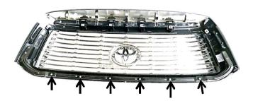
Step 5 Working on work bench. Using a #2 Phillip head screw driver remove 6 factory screws. Set factory grille bracket and hardware aside for later use.
