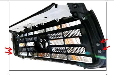
Step 2 Using a 10mm socket locate and remove 2 factory bolts on each side of the factory grille as shown above. Set hardware for reinstallation.
