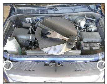
Using a plastic clip removal tool or similar tool remove 2 factory clips circled above.
