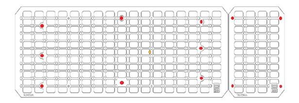
2. With (3/8) .375 drill bit drill holes out for white nut inserts. No, the nut insert will not fit in the hole yet.
