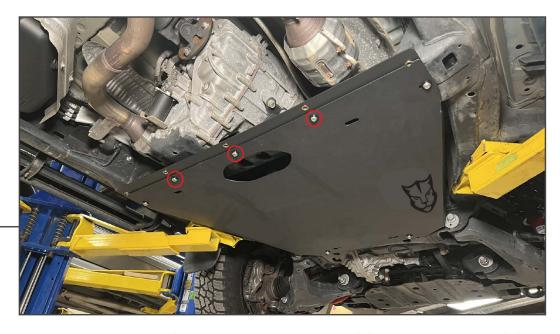
Secure the center skid plate panel to the front skid plate panel using (3) M10 x 20mm bolts, (3) M10 lock washers, and (3) M10 flat washers.
