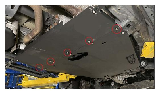
Loosely secure the rear skid plate panel to the center skid plate panel using (5) M10 x 20mm bolts, (5) M10 lock washers, and (5) M10 flat washers into the center skid plate panel threaded inserts.
