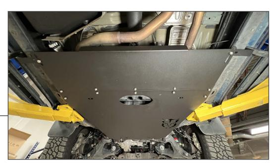
Adjust the skid plate panels for best fit, then tighten all skid plate mounting hardware until secure.
