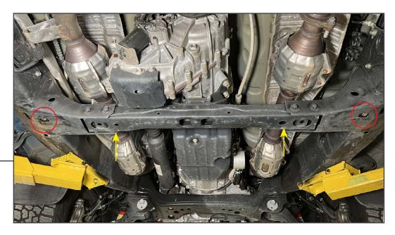
From under the vehicle, insert (2) M10 nut plates into the rear of the vehicle frame under the rear of the transmission.
