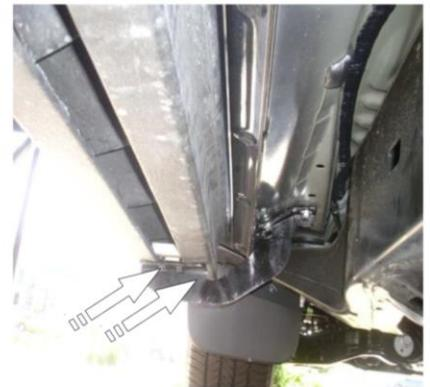
**TORQUE SEQUENCE.** (Fig. 7-a) 8. Perform the following tightening sequence. (a) Torque all body fasteners to 16.3 Lbf-ft (22.1 Nm). (b) Torque all board fastener to 16.3 Lbf-ft (22.1 Nm).
