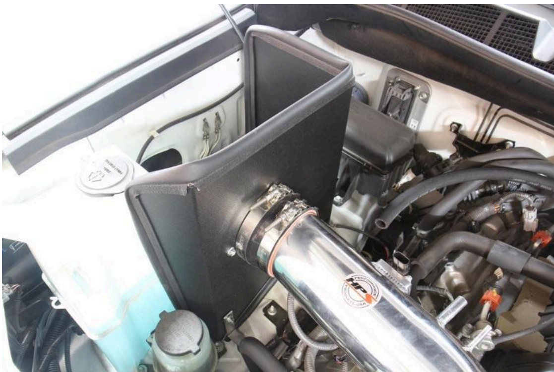
14. Secure the venturi adapter using an M6 washer and bolt on each bolt hole. Secure the pipe once properly positioned.
