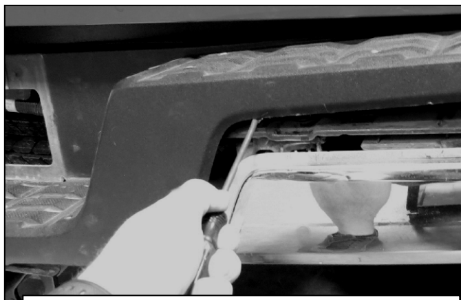
(Fig 6A) Remove center plastic piece on top of the bumper
