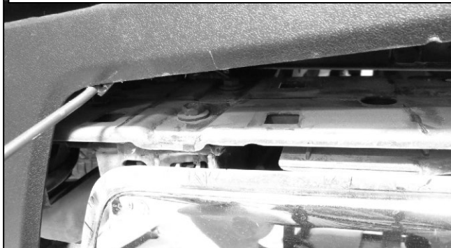
(Fig 6B) Remove factory hardware under the plastic pieces.
