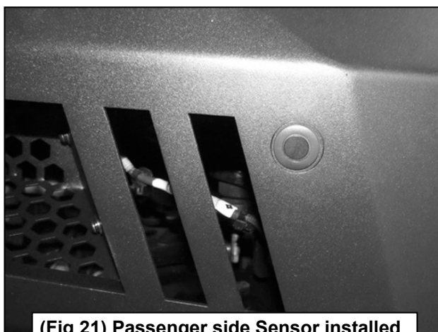
(Fig 21) Passenger side Sensor installed
