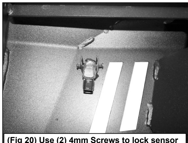
(Fig 20) Use (2) 4mm Screws to lock sensor in place.
