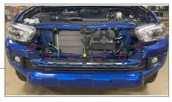
Remove (6) push clips from the bumper. Unplug the connector in the middle of the bumper.
