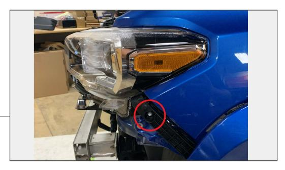
Remove (1) 10mm bolt from the side of the headlight.
