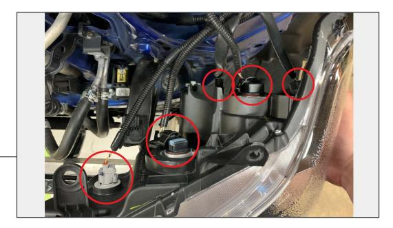
Unplug the (5) connectors from the back of the headlight. Remove headlight from vehicle.
