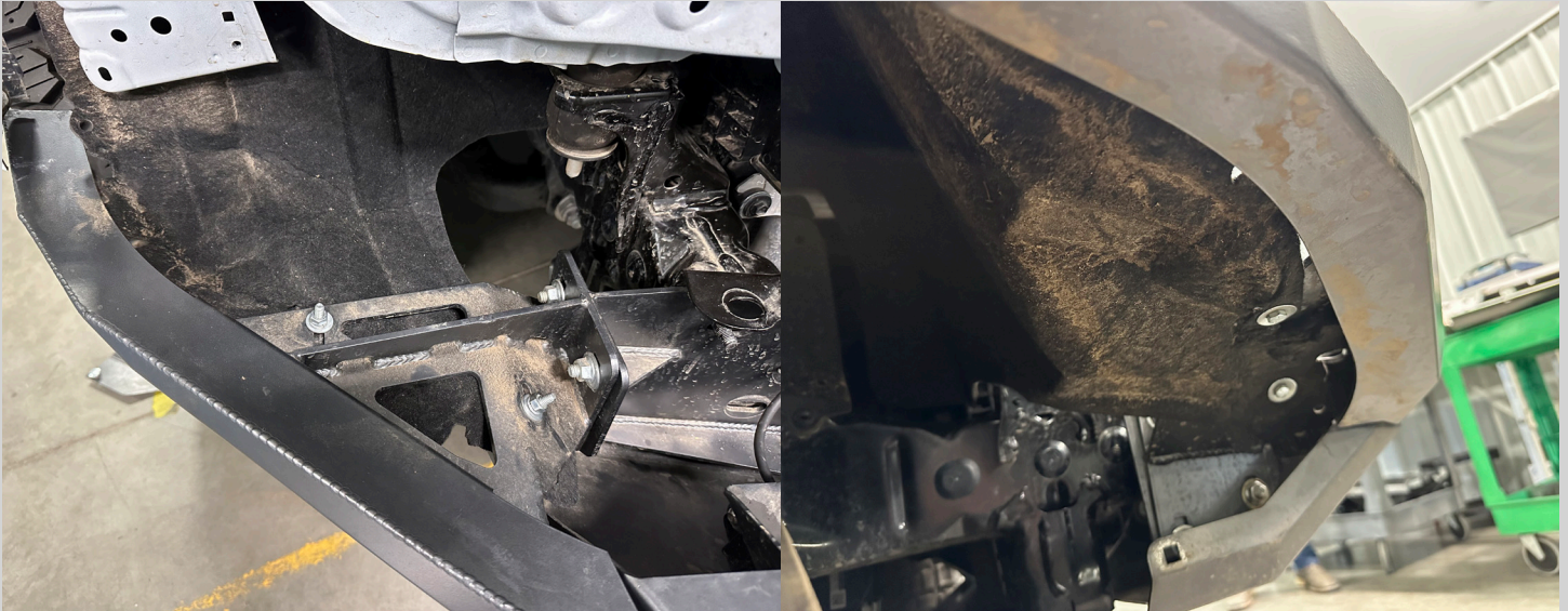
Figure 9: Fender liners secured to the HCSA's using the supplied 1/4" hardware.
