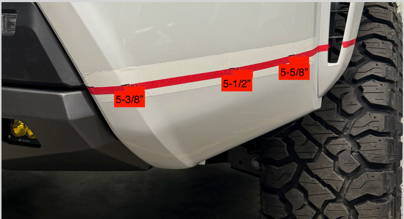
Figure 4: Mark at the lower corner of the black center portion of the bumper cover and 1/2" masking taper connecting the measurement points.
