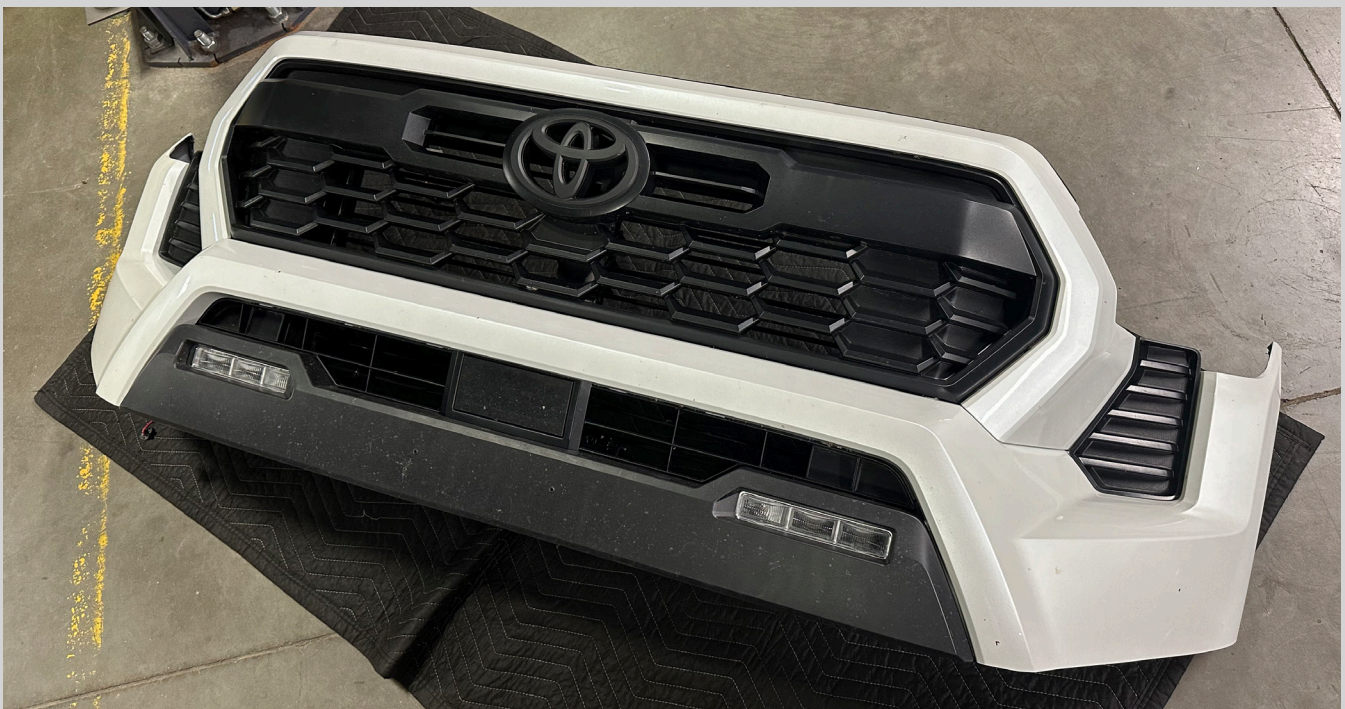
Figure 5: The bumper cover is cut for both the Lo-Pro bumper and High-Clearance Side Additions.
