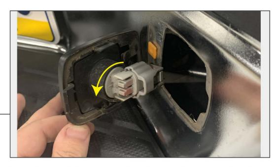
Remove the lens from the bumper. Twist counter-clockwise to remove the connector from the lens.
