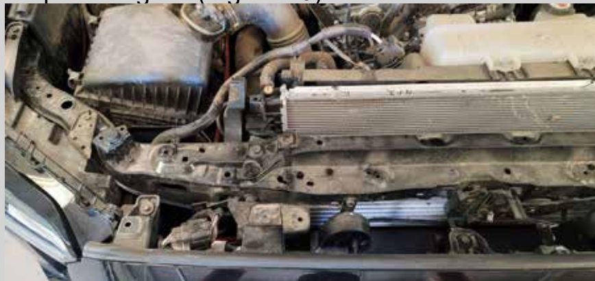
Figure 10: Disconnect the electrical connectors seen in the lower left of the image.
