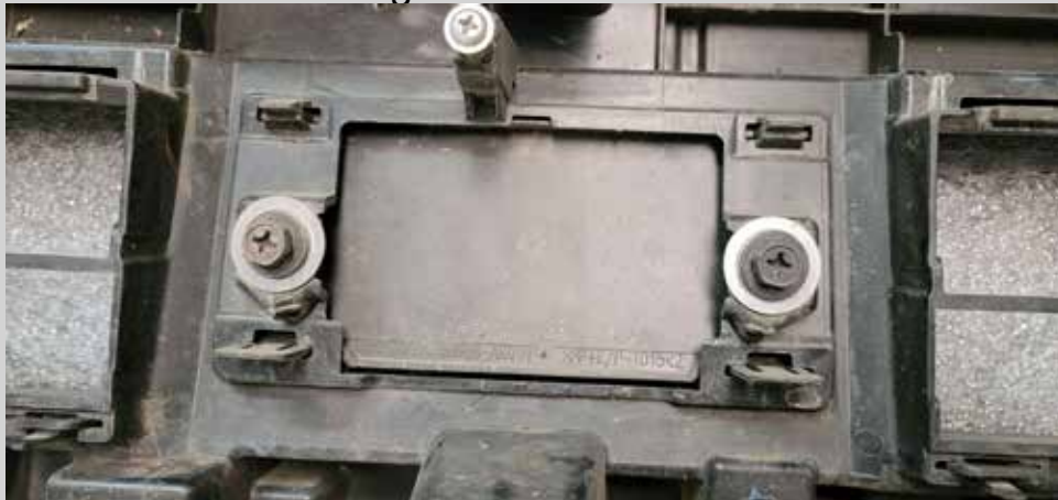
Figure 18: Remove the TSS sensor lens cover.
