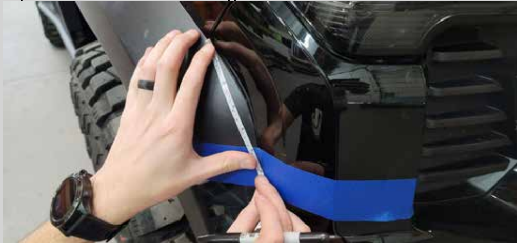
Figure 4: Measure from the point to where the flare and bumper cover meet.
