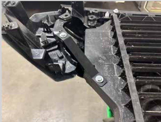
Figure 28: Drill a hole in the shutter frame and bolt the brackets to it.
