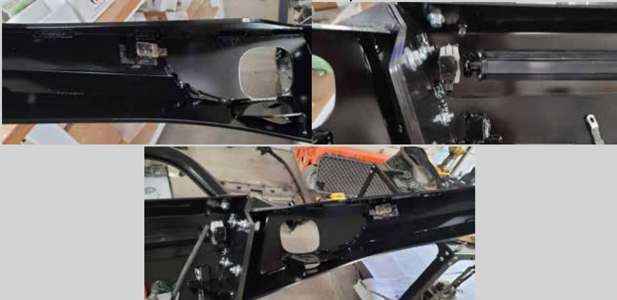
Figure 44: Outer park sensors with plugs facing the bumper center and inner park sensors with plugs facing downward.
