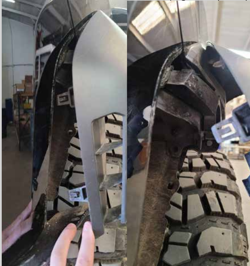
Figure 12: Tabs on the fender flare that need to be depressed to unclip.
