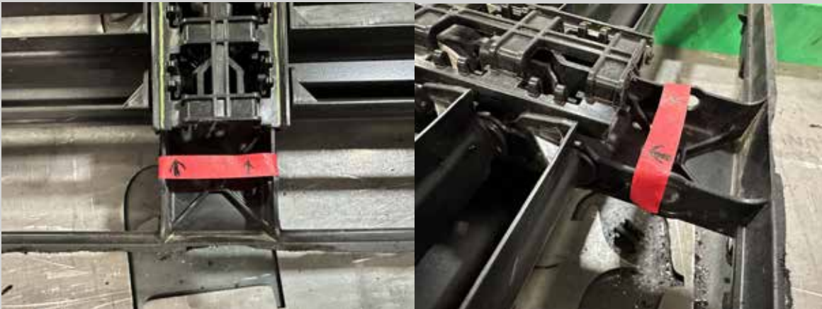
Figure 34: Mark and cut the center just above the pivot point of the fins that were removed.
