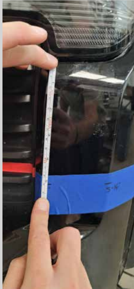
Figure 6: Measure down the inside body line.
