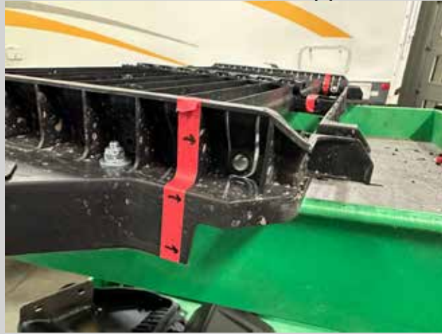
Figure 33: Mark the sides and cut here.
