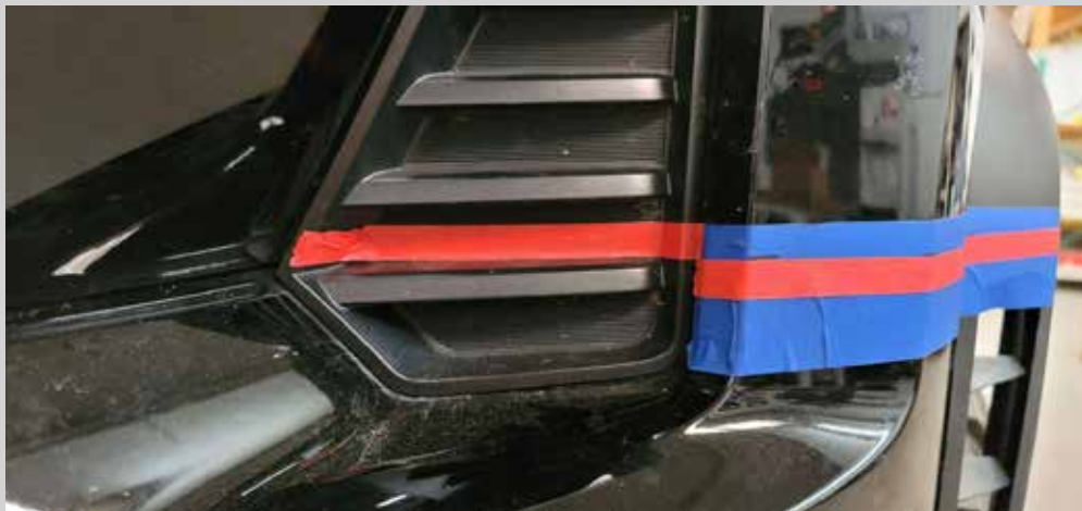
Figure 8: Connect the corner tape line across the black plastic insert to the corner of the grille surround.
