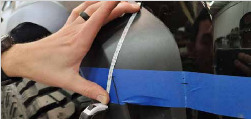
Figure 3: Measure down to the sharp body line on the flare.
