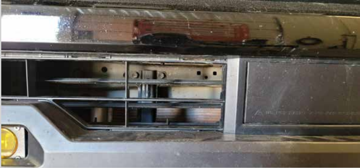
Figure 14: Remove the 2 bolts securing the lower bumper bracket on each side.
