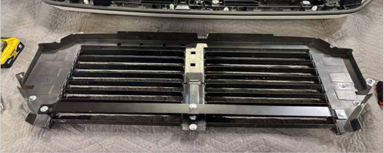
Figure 35: Install the lower grille shutter brace.
