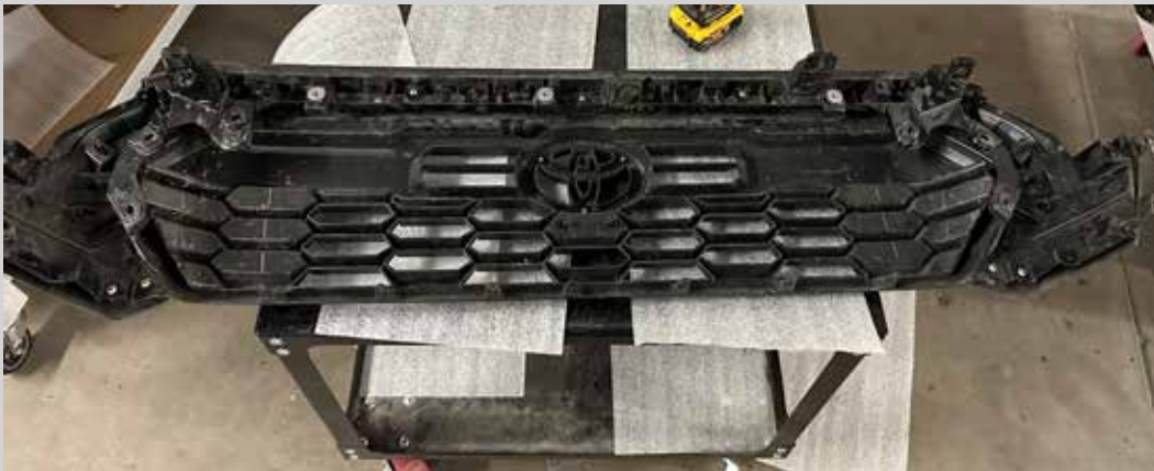
Figure 26: Grille completely reassembled after cutting.
