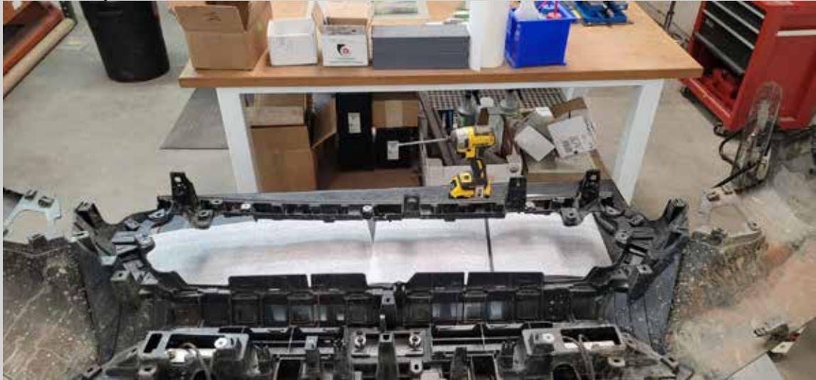
Figure 23: Remove the wiring harness from the bumper cover.
