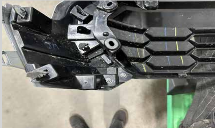
Figure 25: Cut edge hidden by grille surround.
