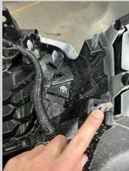
Figure 21: Depress the tabs then push through.
