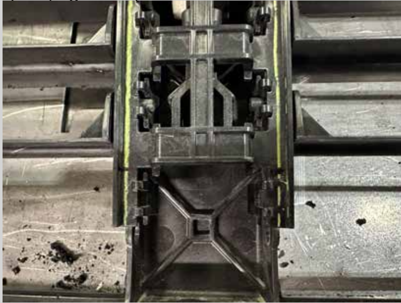
Figure 30: Mark the shutter mechanism to cut off the lowest tabs.
