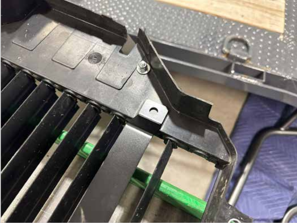
Figure 32: Align the lower support brace as shown and drill the side holes.
