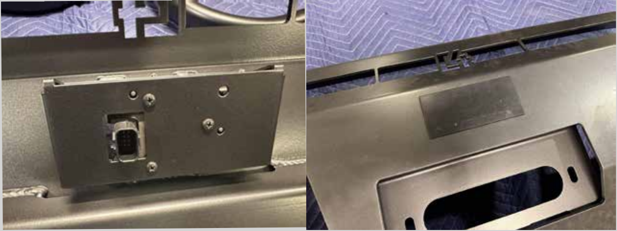
Figure 52: Install the TSS sensor and lens cover.
