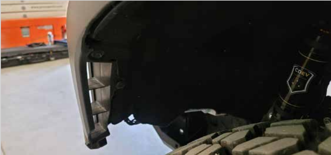
Figure 11: Remove the screws and clips along the front edge of the fender flare.
