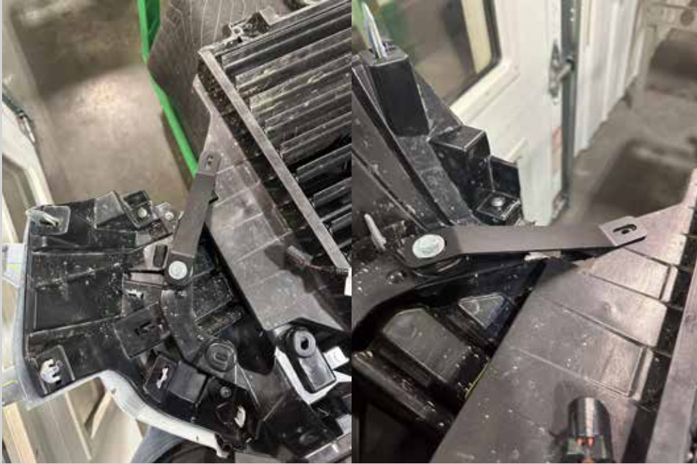
Figure 27: Install the shutter frame support brackets as shown.
