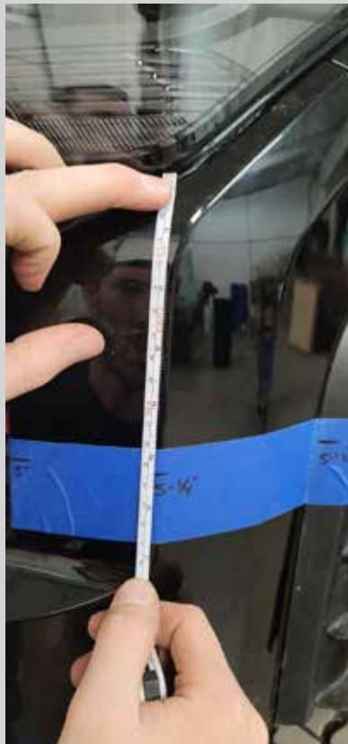
Figure 5: Measure down the corner body line.
