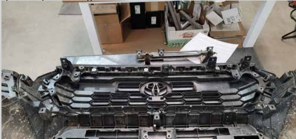
Figure 20: Place the bumper face down to access screws and tabs.
