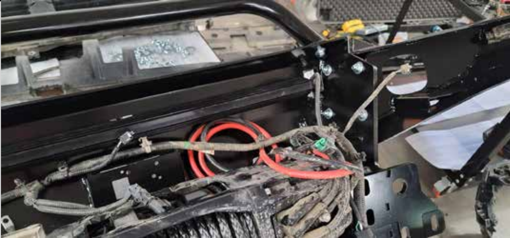
Figure 54: Route the wiring harness to the sensors and fog lights.
