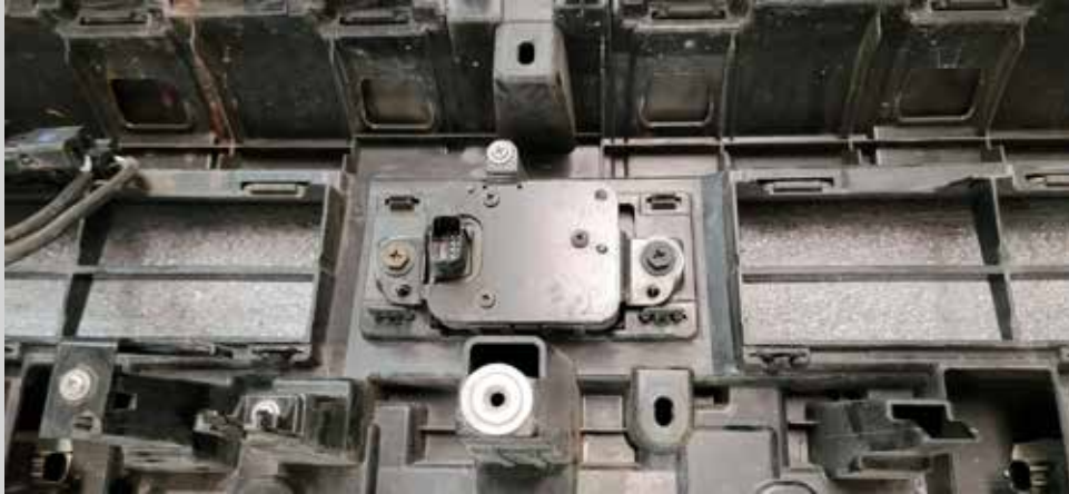
Figure 17: Remove the TSS sensor.
