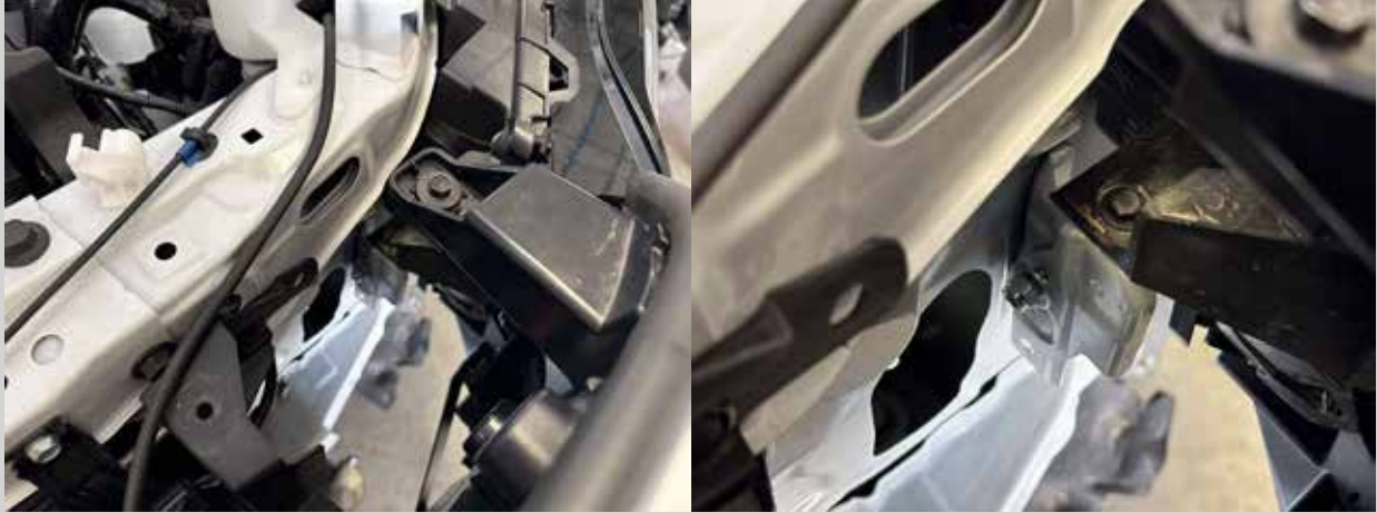
Figure 55: Start the hardware for the lower grille support.
