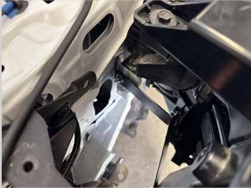
Figure 56: Lower grille support L-bracket installed.
