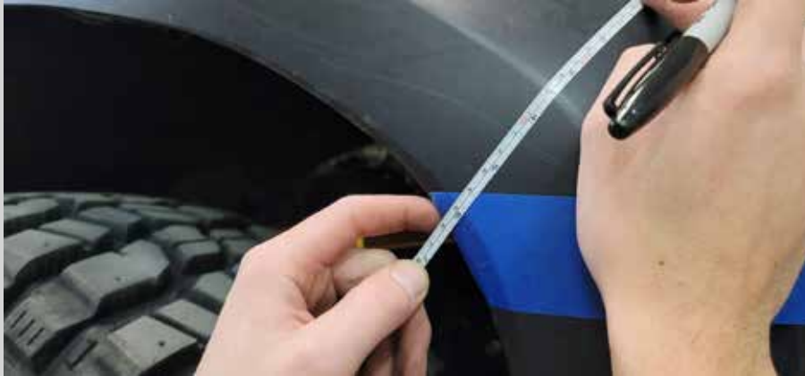
Figure 2: Measure downward to the edge of the flare.
