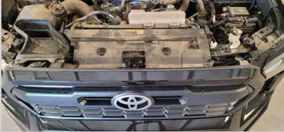
Figure 9: Remove the radiator cover and the air intake duct.
