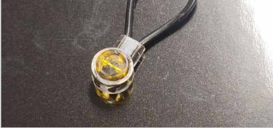
Figure 51: Wire splice properly crimped.
