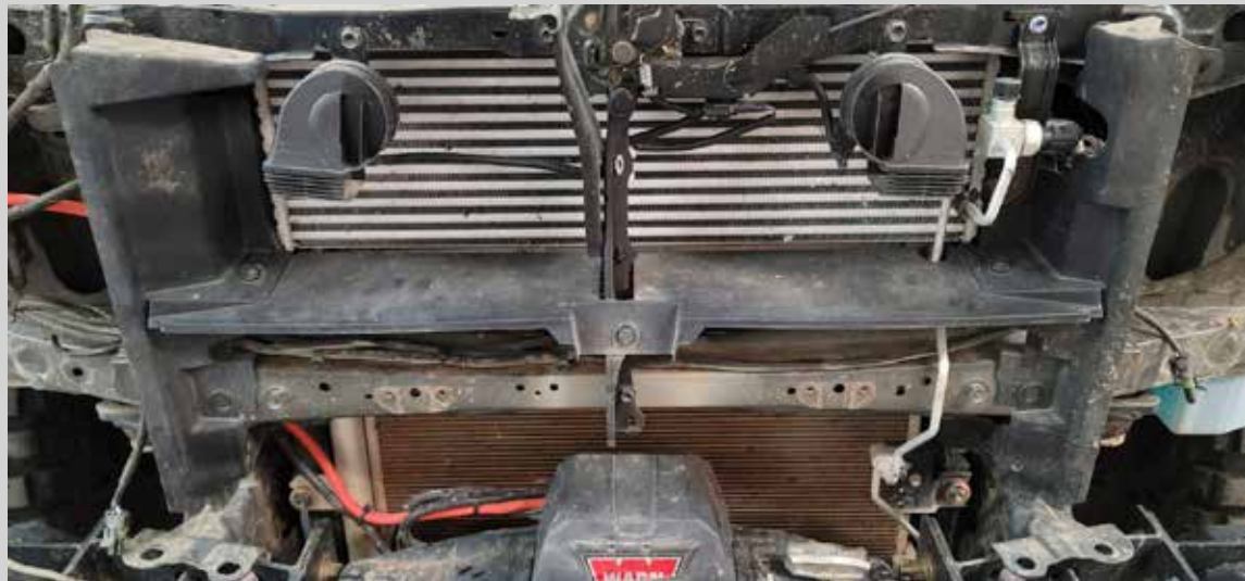
Figure 15: Lower brackets removed. (Bumper cover removed for view)
