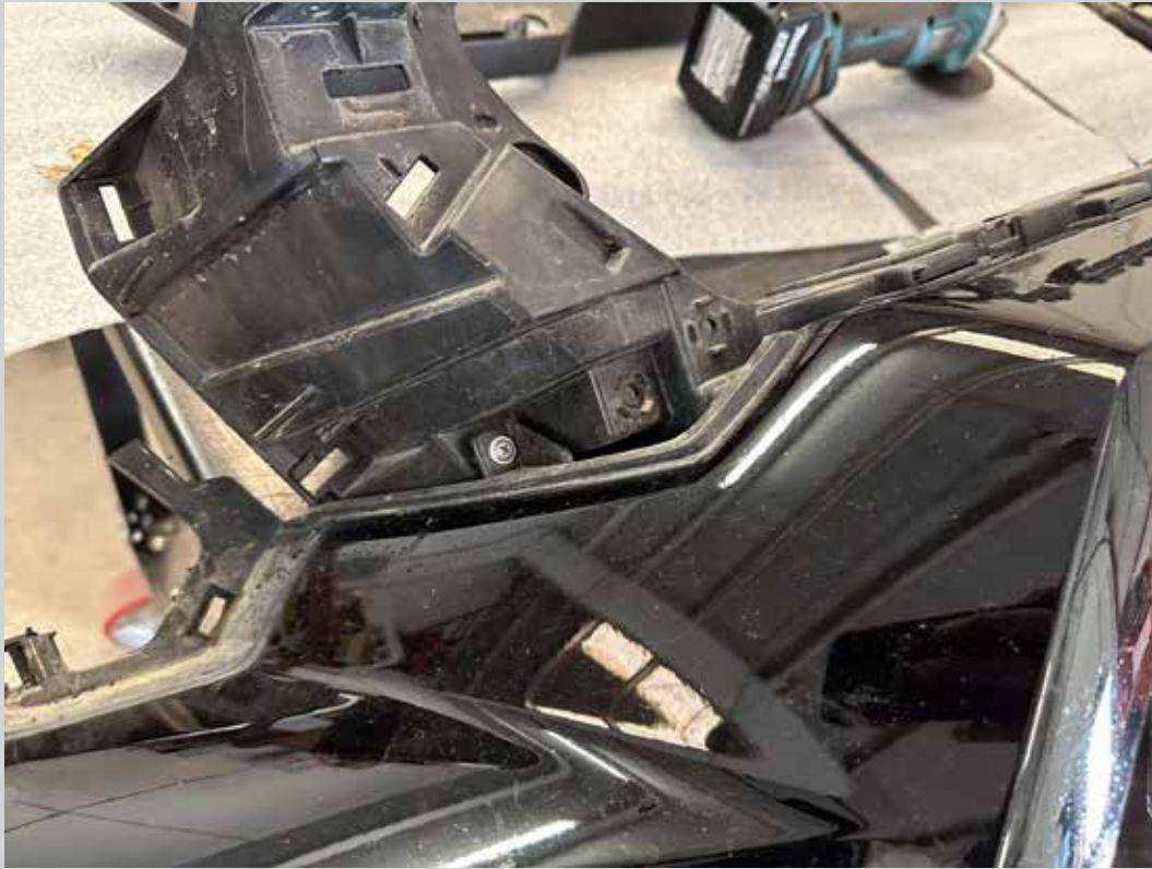
Figure 22: Remove the screw on the front on each side.
