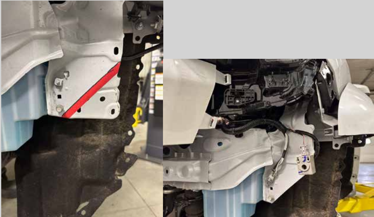
Figure 36: Left, mark and cut the structure. Right, reattach the ground wires and lock beeper.
