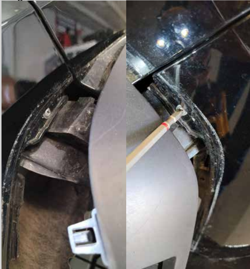
Figure 13: Remove the screw behind the fender flare.
