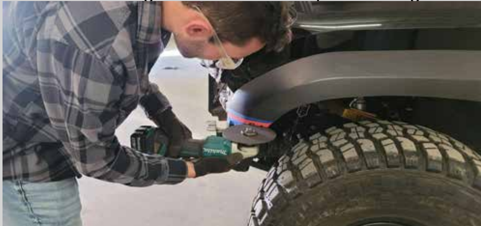
Figure 38: Cut the bumper cover and the fender flares.
