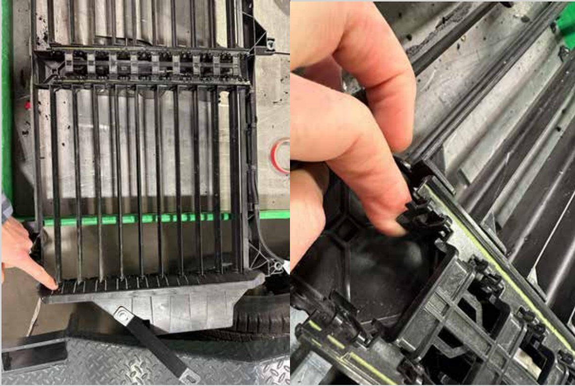
Figure 29: Remove the bottom shutter fin on each side.
