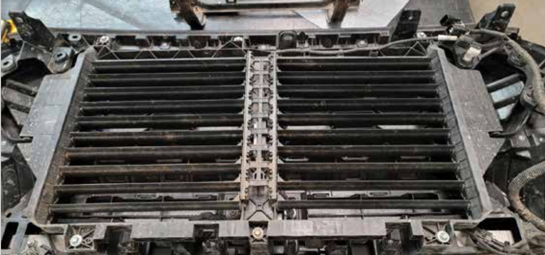
Figure 16: Grille shutters to be removed.
