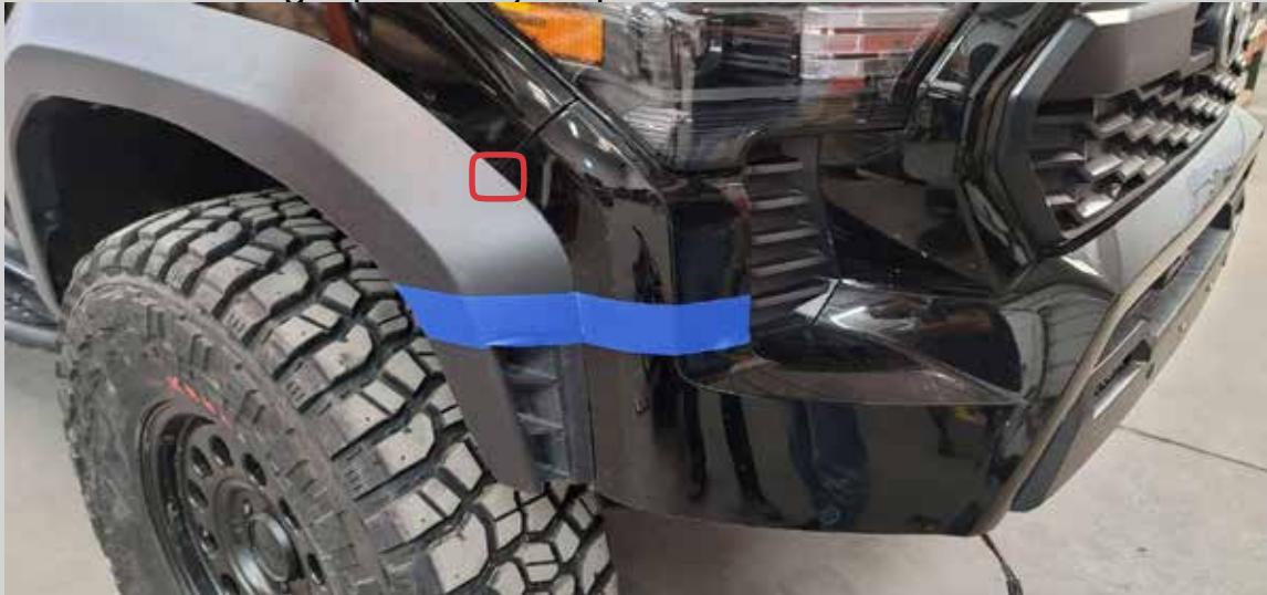
Figure 1: Place a piece of masking tape as shown. The circled point is where the measurements for the flare will start from.
