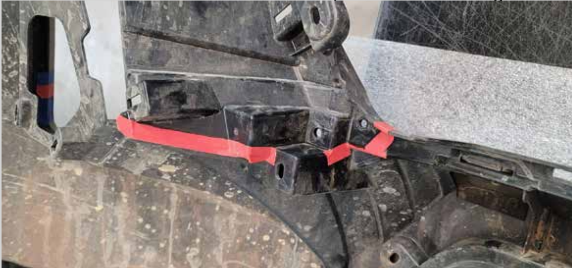
Figure 24: Mark the grille frame on each side as shown.
