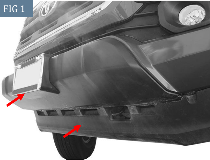
(Fig 1) Remove the license plate and air dam from front bumper cover
