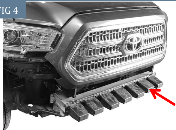
(Fig 4) Remove plastic impact pad (arrow), NOTE: Pictured with plastic bumper cover removed for instruction purposes only, it is not necessary to remove bumper cover
