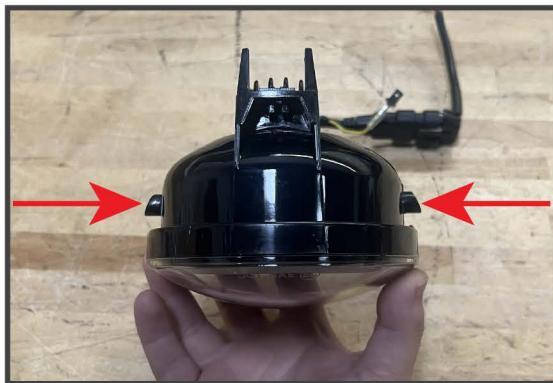
3. Fit the included alignment retainer to the lower portion of the fog light mounting area. This must be installed before the fog light.
