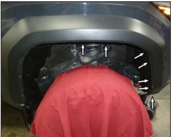
2. Inner fender apron bolt and clip locations.
