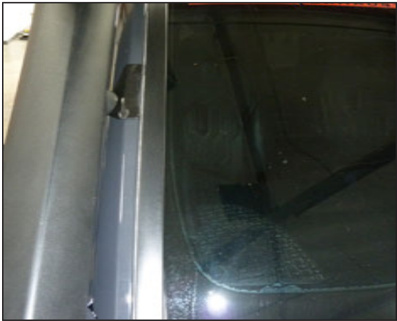
26. Reinstall the passenger side windshield trim.
