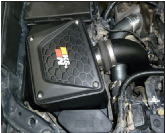
30. During extreme conditions the optional factory fresh air block-off and K&N lid block-off can be installed to force all intake air to pass through the snorkel if desired.
