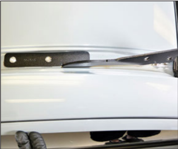
18. Align the snorkel mounting bracket with the inserted nuts and secure with the provided hardware. NOTE: Be sure to apply the provided thread locker to the mounting bolts before installation.
