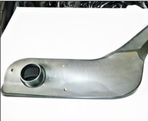
20. Peel the paper backing off the cushion pad and then apply the pad to the snorkel as shown.
