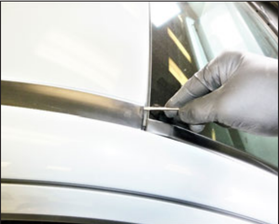
16. Vehicles that are equipped with a factory TOYOTA roof rack, skip to step #20. Using a small screw driver or similar device, pry up the roof trim to expose the inserted nuts in the roof channel.
