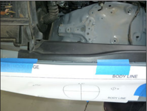
12. With the 2nd template with no holes cut out, tape to the front fender as shown. Using the template guide, mark the four locations in the fender that will be drilled with a center punch or similar device. NOTE: The fender sheet metal is thin, light tapping is all that is needed to mark the hole location.
