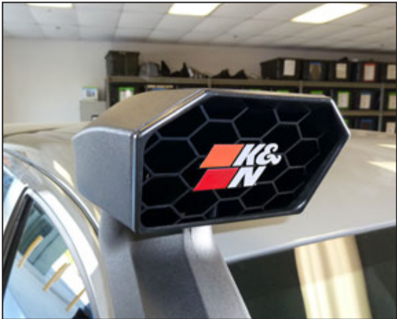
29. Install the snorkel scoop onto the snorkel and secure with the provided hose clamp.
