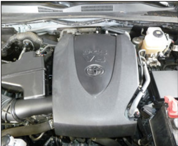
38. Reinstall the engine cover.
