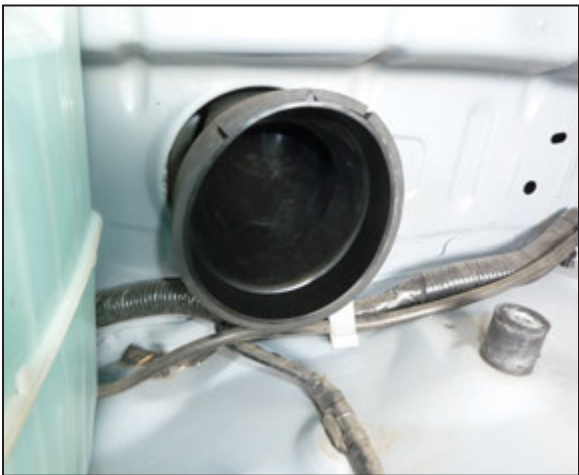
34D. Install the flexible spacer into the flexible duct as shown and then the AIRAID air filter housing can be installed.
