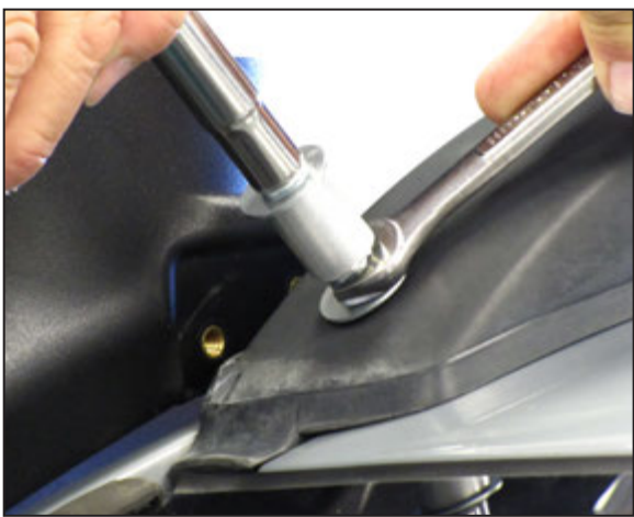
27. Using a 9/16" wrench to hold the nut and a 10mm socket and ratchet to tighten the bolt while applying downward pressure on the bolt. This compress the Rivnut and grip the plastic of the roof rack. Tightening force will be high initially and then lessen until the Rivnut is set. Force will ramp up again once set, do not over tighten.
