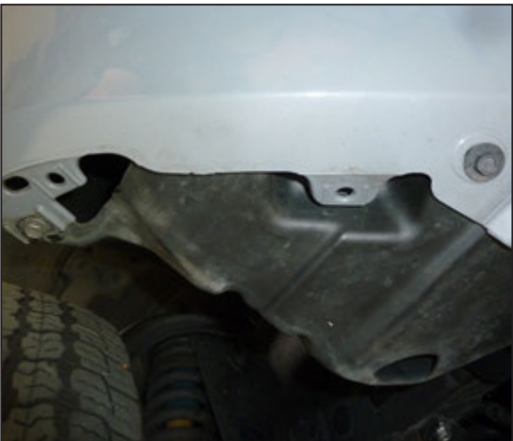
31. Replace the two inner fender retaining clips with the clips provided and then reinstall the two factory screws.
