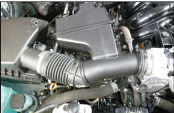
36. Reinstall the intake tube and secure with the factory hose clamps. Reconnect the vent lines.
