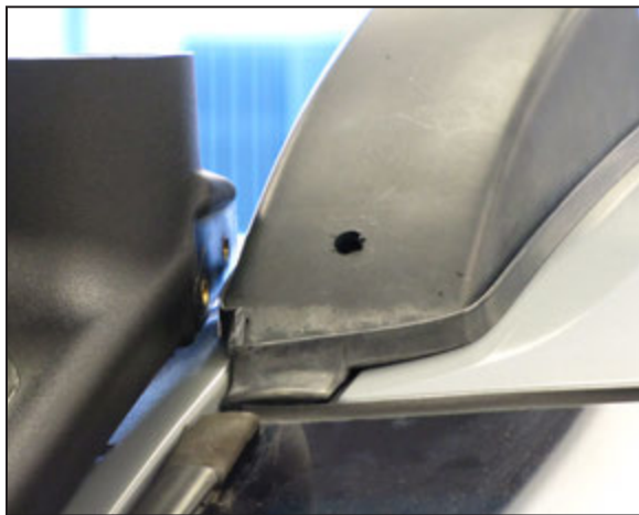
25. Drill a 1/8" ID pilot hole into the marked location on the roof rack and then drill a 25/64" ID hole.
