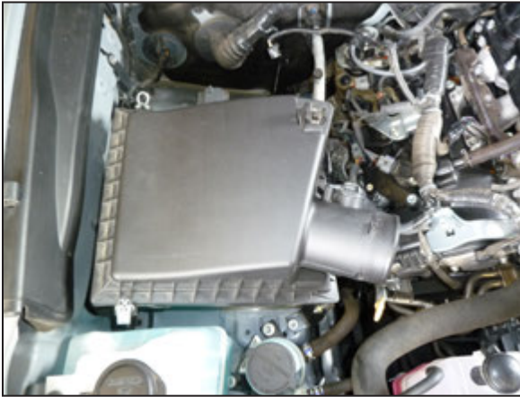
35. Install the air filter and upper housing to flexible spacer and secure using provided clamp.
