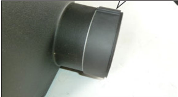
34A. if using an AIRAID intake kit (AIR-511-309), install the provided flexible spacer onto the AIRAID filter housing inlet as shown. Using a marker, draw a line around the inlet using the spacer as a guide.
