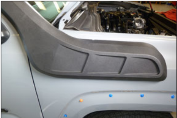
24. On vehicles equipped with a factory TOYOTA roof rack, install the snorkel onto the fender with the provided top bracket. Mark the location for the hole to be drilled into the roof rack.
