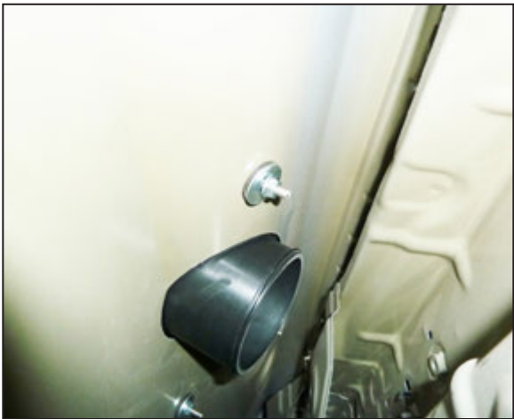
22. Secure the snorkel to the fender with the provided rubber washers, fender washers and flange nuts.
