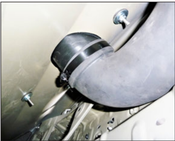
29. Install the snorkel scoop onto the snorkel and secure with the provided hose clamp.
