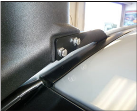
23. On vehicles without a factory TOYOTA roof rack, install the snorkel onto the fender and secure it to the top mounting bracket with the hardware provided.
