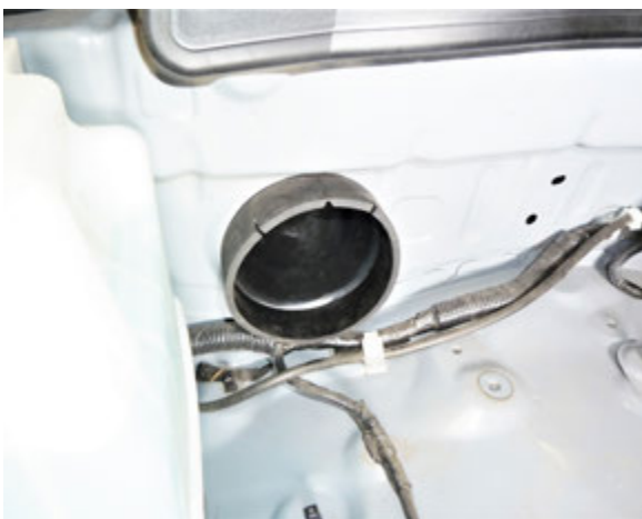
30. Install the flexible duct onto the snorkel and through the opening into the engine compartment. Adjust for best fit and then secure it to the snorkel with the provided hose clamp.
