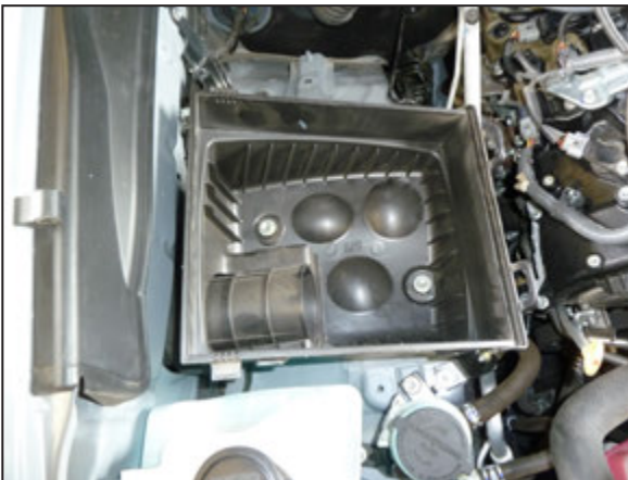
33. Reinstall the lower air filter housing and secure with the factory hardware. Secure the snorkel duct to the air filter housing with the provided hose clamp. NOTE: It may be necessary to move the washer bottle to gain access and tighten the hose clamp.
