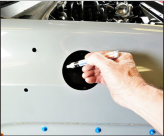
15. Apply a coat of paint to the inside of the holes drilled to prevent corrosion.
