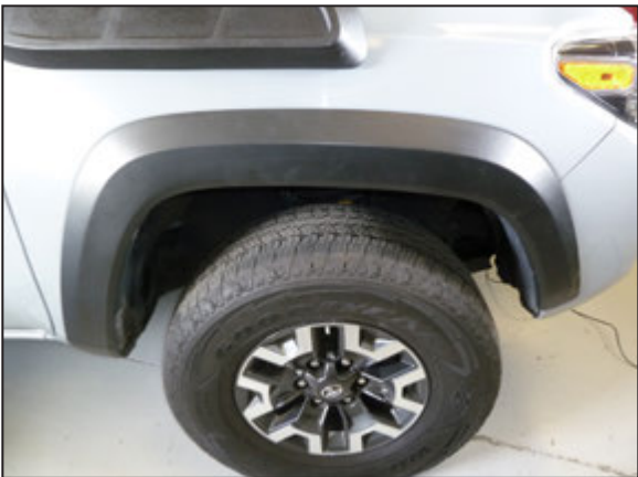
32. If equipped with fender flares and or mud flap, reinstall them onto the fender.
