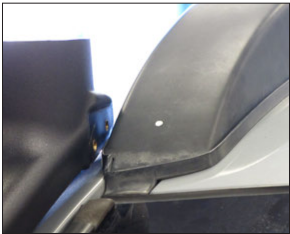
24. On vehicles equipped with a factory TOYOTA roof rack, install the snorkel onto the fender with the provided top bracket. Mark the location for the hole to be drilled into the roof rack.
