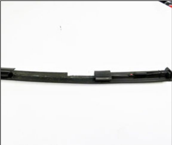
19. Set the roof trim back in position and note where the bracket interferes with the trim. Using side cutters or a razor blade, trim the roof trim so that it will lay flat back into the channel and around the bracket.
