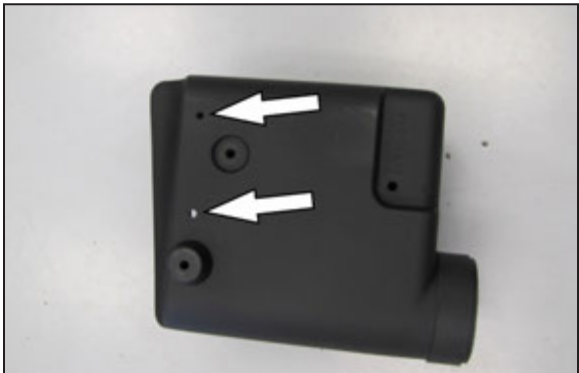
34C. Drill two 3/8" ID holes into the bottom of the AIRAID air filter housing for water drainage.
