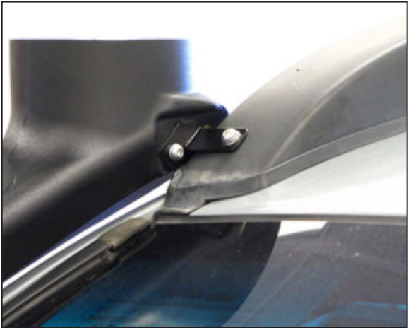
28. Install the upper mounting bracket and secure with the provided hardware.
