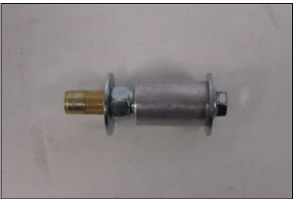
26. If a Rivnut setting tool is not available, assemble the provided hardware as shown to install the Rivnut. NOTE: The nut passes over the threads of the bolt, it does not thread on.
