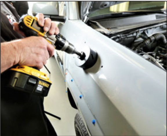
14. Drill three 5/8" holes for the snorkel mounting location and using a 4" hole saw, drill the 4" hole for the air duct. NOTE: the 4" hole will be drilled through different angled surfaces, use caution while drilling to not distort the remaining sheet metal.
