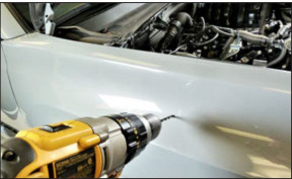
13. Drill a 1/8" pilot hole in all four locations to be drilled.
